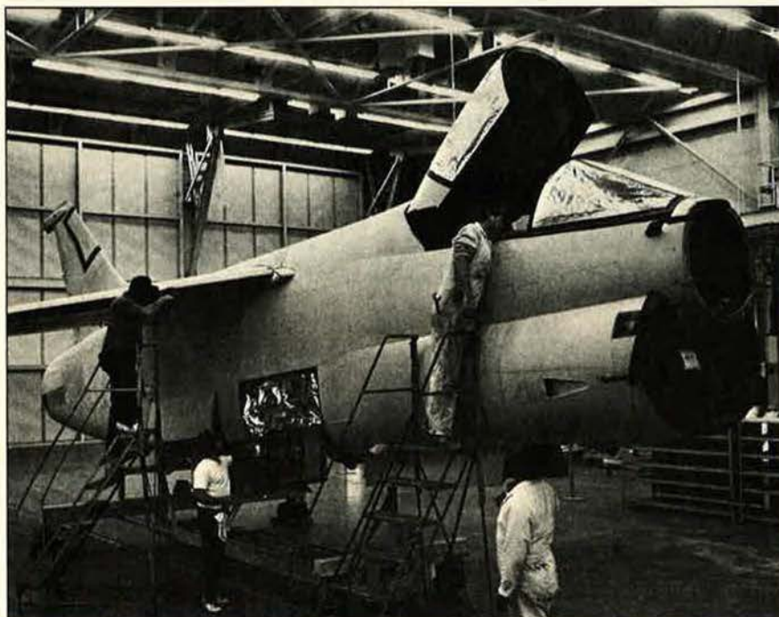
The first of two LTV A-7D attack aircraft to be modified to the "A-7 Plus," or as it is officially called now, YA-7F, configuration is being stripped down by workers in the company's Dallas, Tex., facility. The two aircraft will be lengthened, reengined, and equipped with improved avionics as part of a $133.6 million effort.
