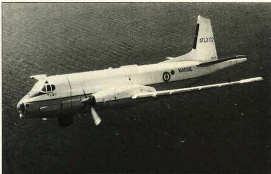
The French Ministry of Defense has authorized the production of the Atlantic 2, of which forty-two will be acquired by the French Navy. While the airframe and engines are identical to those of the predecessor Atlantic 1, the equipment for antisubmarine and antisurface warfare is entirely new. The Atlantic 1 was selected by NATO in 1958 as its maritime aircraft and was designed specifically for that mission.
