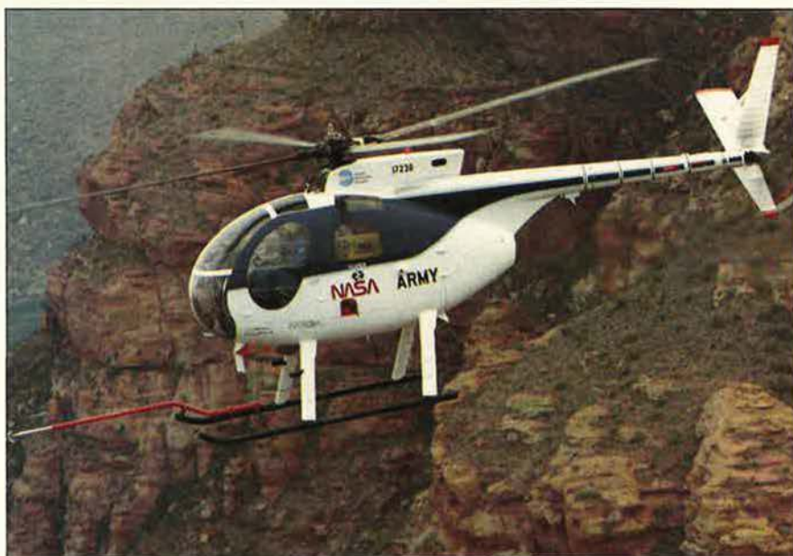
Hughes Helicopters, Inc.'s Higher Harmonic Control (HHC) aircraft undergoes flight-testing of its computerized vibration-control system at the company's Mesa, Ariz., facility. Demonstrated has been a reduction of eighty percent or more in fuselage vibrations at cruise speeds and during selected maneuvers. This should provide a boost for sensitive avionics and weapon systems, a reduction in maintenance, and a more stable weapons platform. HHC is a joint Army/NASA program.
