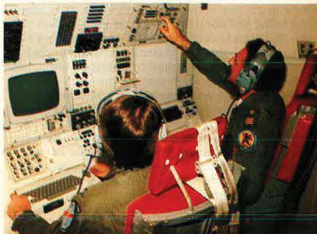
A technician checks a Joint Tactical Information Distribution System (JTIDS) terminal aboard a NATO E-3A aircraft. An Enhanced JTIDS System (EJS) is now under development.
