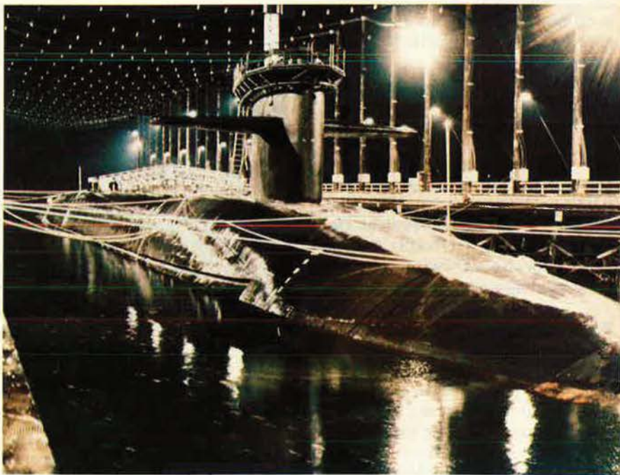
In the surrealistic setting of a magnetic silencing facility, the ballistic missile submarine USS Ohio undergoes a change in the giveaway "signature" it had acquired from the earth's magnetic field. A major requirement of US strategic C 3 is keeping the National Command Authorities constantly in touch with such nuclear-retaliation SSBNs.
