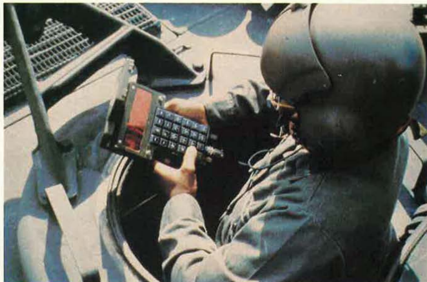
A US armored vehicle commander uses a Navstar receiving unit to establish his ground position. Navstar Global Positioning System (GPS) satellites play a vital role in US command control and communications.
