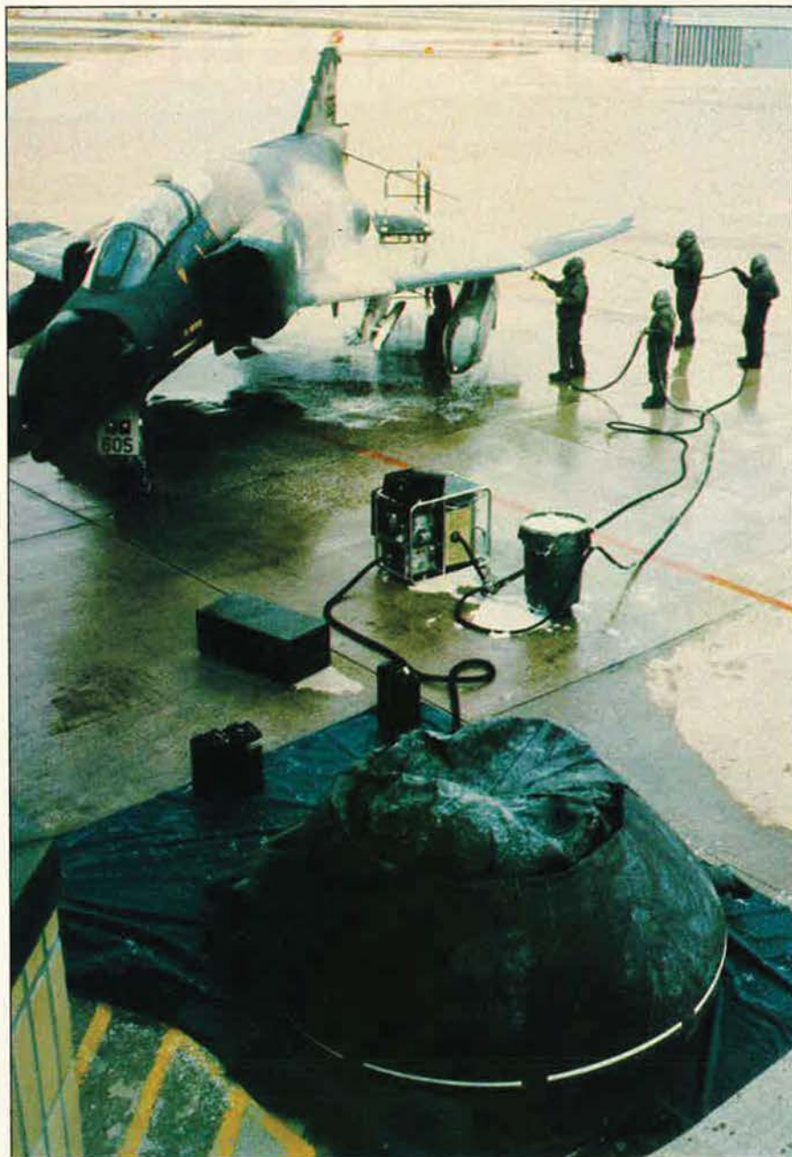
A new, lightweight decontamination system, shown here during a recent chemical defense exercise at Lambert Field in St. Louis, Mo., is currently being distributed to US bases overseas. AFSC's Aeronautical Systems Division will acquire 1,500 to 1,600 of the systems for eventual use at CONUS bases. In the foreground is the system's 1,580-gallon-capacity, collapsible, fabric tank. See item.
