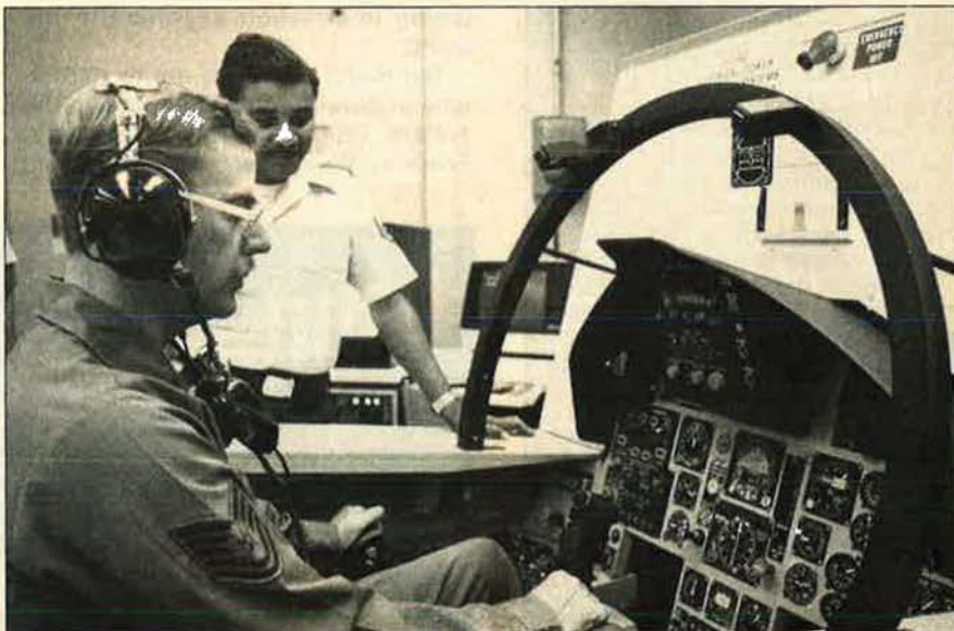
Seated in a student cockpit trainer, MSgt. David Geer performs "hands-on" maintenance training procedures for the F-15's electrical power, lighting, and engine operative systems. Honeywell Training and Control Systems Operations, under contract to McDonnell Aircraft Co., St. Louis, Mo., delivered the first of two Simulated Aircraft Maintenance Trainers for the F-15 Eagle to Luke AFB, Ariz., late in 1983. In addition to the cockpit, the trainer includes a master simulation control console.
