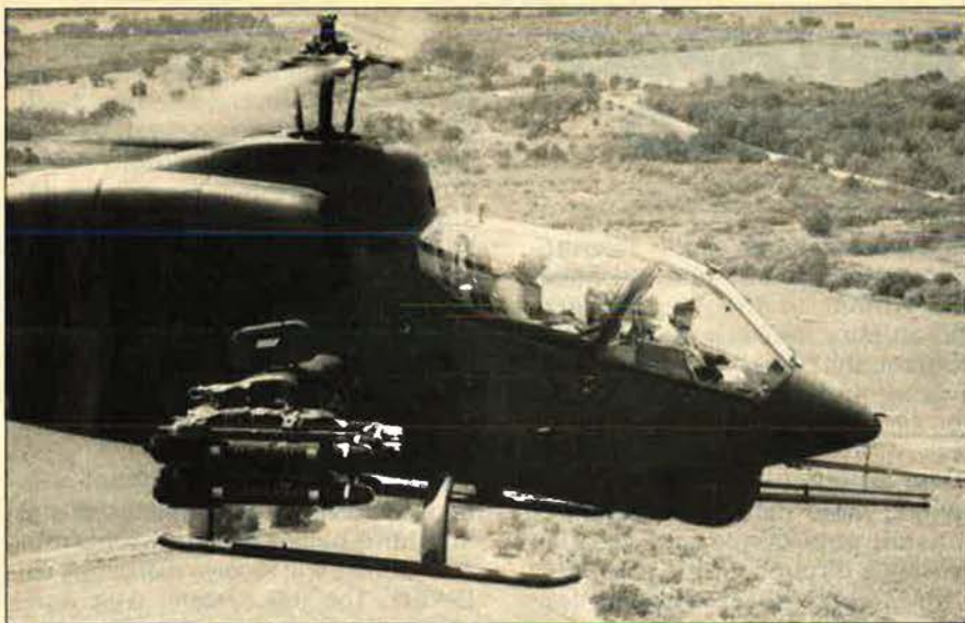
Bell Helicopter has test-flown its AH-1J Sea Cobra for airworthiness, including airframe compatibility with Rockwell International Missile Systems Division's Hellfire antiarmor missile. Flight load and vibration tests, covering the complete performance envelope, have been completed. Missile firings are planned for early 1984. The AH-1J and Hellfire are part of a US Marine Corps program.
