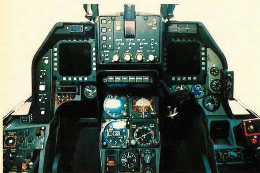
The AFTI/F-16 cockpit exemplifies USAF's emphasis on making pilots more productive and comfortable. Among major changes are two multipurpose displays and a wide field of view head-up display.
