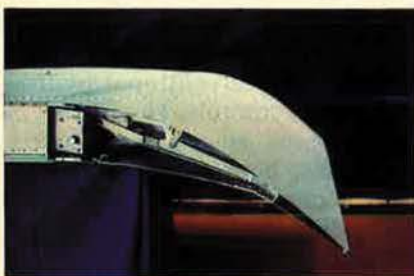
Mission-adaptive wing, using electronically controlled internal mechanisms to change its always-smooth shape (left) in flight, should greatly enhance the performance of future aircraft. The first of these variable-camber wings, built by Boeing, were recently installed (above) on an Advanced Fighter Technology Integration (AFTI) F-111 at NASA's Dryden Flight Research Facility, Edwards AFB, Calif., for testing beginning late next summer.
