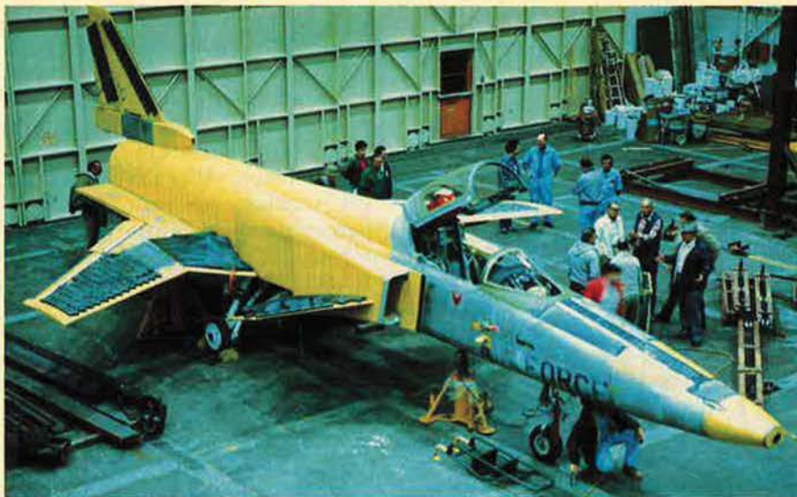
Grumman Corp.'s X-29 forward-sweptwing demonstrator aircraft takes shape at Grumman's Bethpage, N. Y., facility. Under Defense Advanced Research Projects Agency (DARPA) auspices, the X-29 will test the use of forward canards as the main control surfaces.
