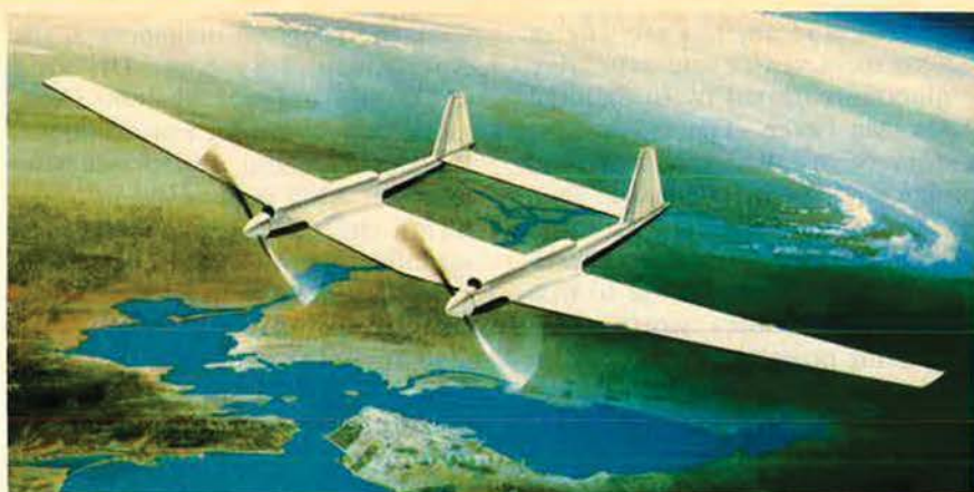
With a wingspan of 267 feet and takeoff weight of 40,000 pounds, Lockheed's proposed high-altitude drone is intended for elint and other military missions. Dual-cycle turbojet/turboshaft engines, burning liquid hydrogen fuel, would provide twenty-four-hour endurance.
