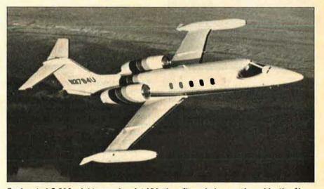
Designated C-21A, eighty new Learjet 35A aircraft are being purchased by the Air Force as replacements for part of MAC's aging fleet of CT-39s. First delivery is expected early in 1984. As a light transport, the C-21A will have a crew of two and seat seven passengers.
