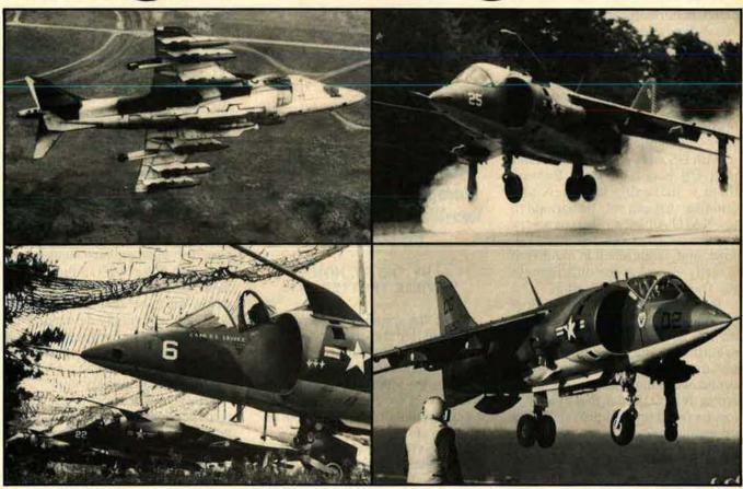
It's the unique vectored thrust of the Rolls-Royce Pegasus engine which gives the new Harrier II/AV-8B its unsurpassed basing flexibility and outstanding speed of response.
