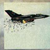
MW-1. Multipurpose weapon system to be used on the Tornado.
