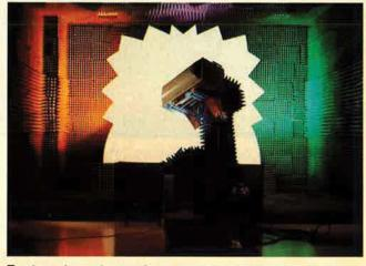
Testing phased array in compact antenna range.
