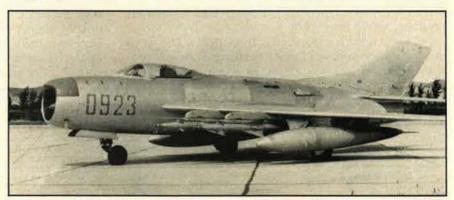
About 3,000 J-6s and variants make up a large part of the Chinese fighter force. The basic design is derived from that of the Soviet MiG-19.
