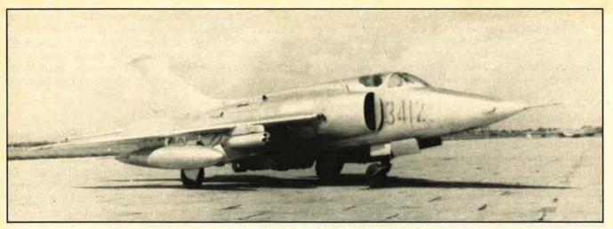
The Q-5, the export version of which is referred to as A-5, is a Chinese-designed ground-attack fighter based on the MiG-19.
