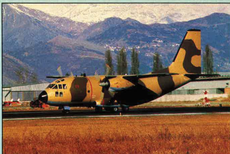
Aeritalia G222 twin-turboprop general purpose transport of the Libyan Air Force, with Tyne engines
