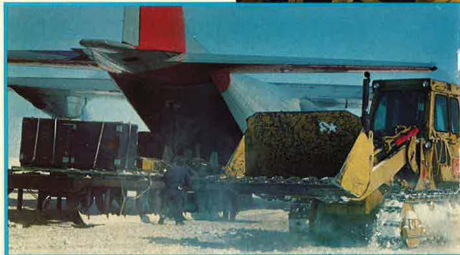
ABOVE: Pallets are pushed onto a giant sled and pulled by a snow-going tractor.
