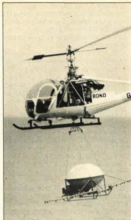
Britain's Rotortech Ltd. has developed this helicopter-borne spraying system that uses concentrated dispersants to fight oil spills. It can be assembled, loaded, and on its way in less than ten minutes, according to officials.
