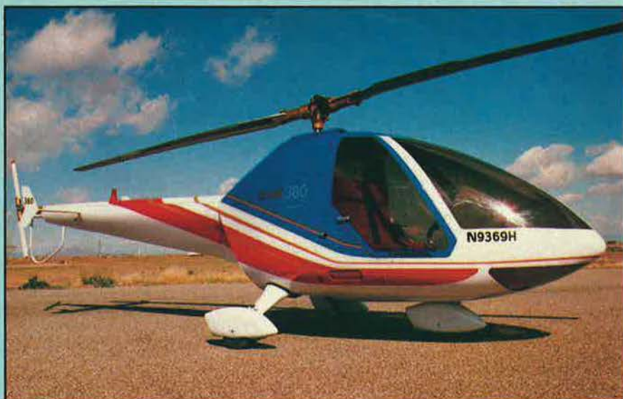
Hillman Model 360 three-seat light helicopter (Avco Lycoming HIO-360-C1A engine)
