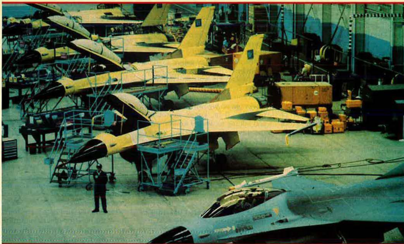
Many panels of the F-16, seen here on the General Dynamics production line at Fort Worth, are made of composite materials. Continued progress in composites will lead to stronger airframes in the future, and will allow economical manufacture of complex surfaces.
