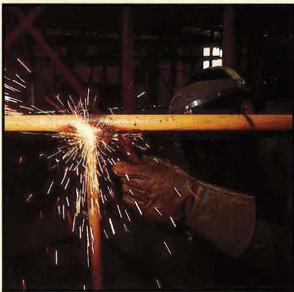
LEFT ABOVE: A1C Lewis Irvin of the active-duty 436th Aerial Port Squadron uses a hand-held computer terminal to check in cargo. (USAF photo by Skip Ruiz) LEFT: In the welding shop, TSgt. Garland Dula, an ART with the 512th FMS, makes sparks fly during oxyacetylene cutting. ABOVE: Working on a C-5 tail assembly is TSgt. Ray McCloskey, an ART with the 512th Organizational Maintenance Squadron. (Photos by TSgt. Kevin Heslin)
