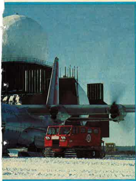
LEFT: The radar station at DYE-2 stands seven stories high, dwarfing one of the men who has duty there. ABOVE: Engines remain running during unloading to avoid restart problems.
