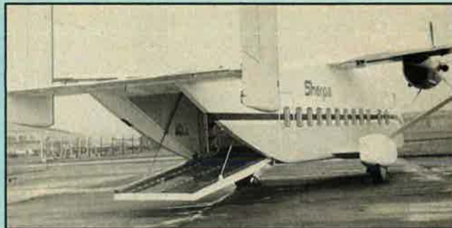
New rear ramp and roller conveyors facilitate loading into the large-section hold
