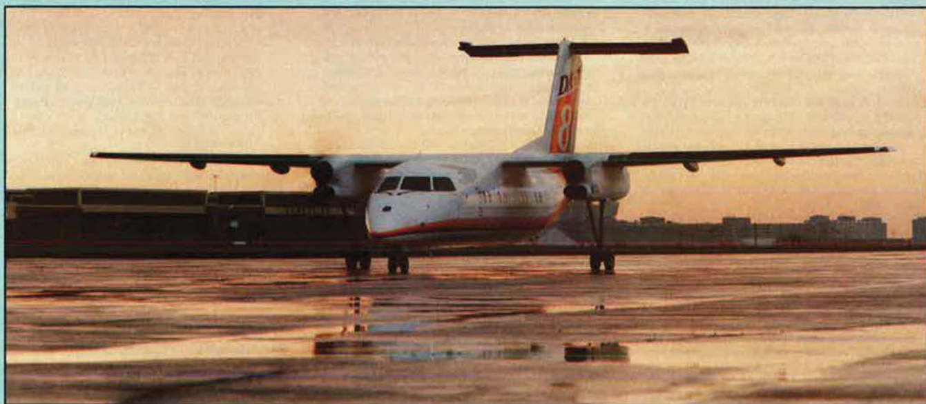
Prototype de Havilland Canada Dash 8 (two Pratt & Whitney Aircraft of Canada PW120 turboprop engines)
