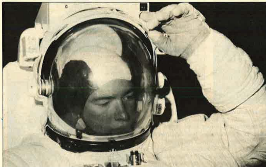
A miniature television camera peering over the helmet of Astronaut Joseph Allen's spacesuit will give viewers on earth a glimpse of the scene during a space walk scheduled for Orbiter Columbia on its STS-5 mission. The first operational flight of the Space Shuttle also calls for the deployment of two communications satellites.
