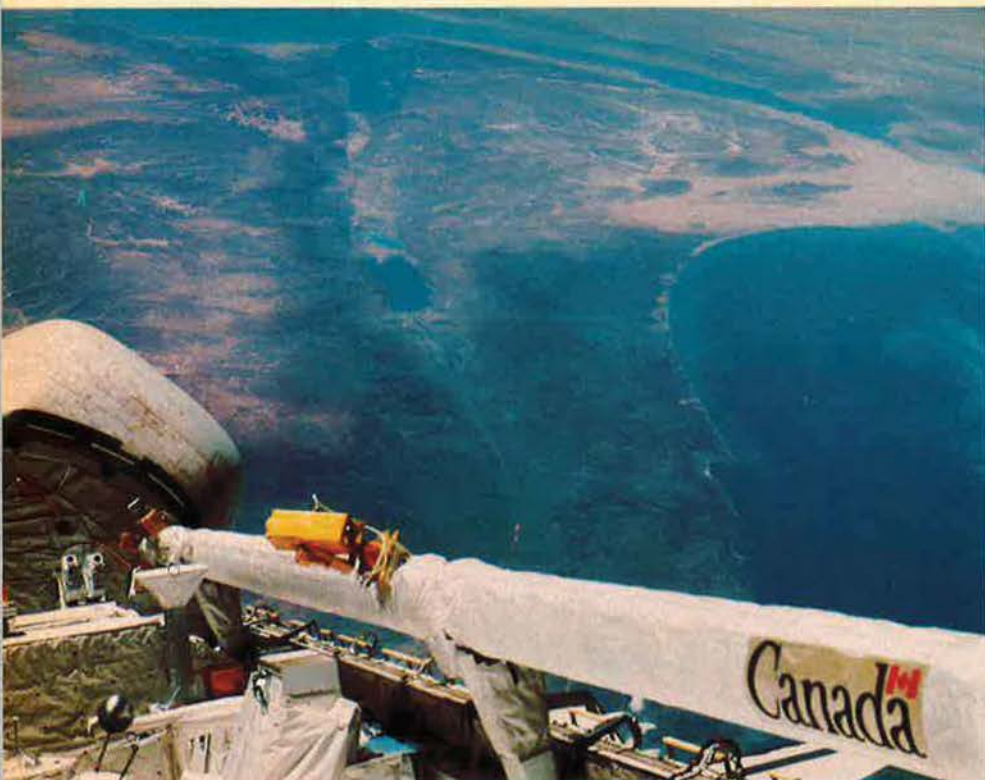
Above, a southerly view from Orbiter Columbia reveals a small portion of the vehicle's aft section and the fifty-foot-long, Canadian-built remote manipulator system arm. The Mediterranean Sea is at the right foreground and other areas of the Mideast can be identified. Below, Columbia enters the Vertical Assembly Building at KSC for mating with solid rocket boosters and external tank. At Vandenberg these components will be joined vertically on the launch pad.
