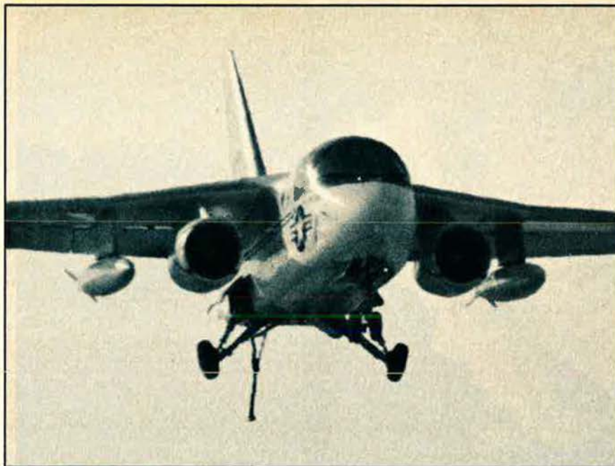
S-3A Viking antisubmarine aircraft approaches for landing aboard USS Forrestal (CV 59). Admiral Miller suggests that S-3As could control critical chokepoints from land bases, operated by USAF crews. S-3A is a four-engine aircraft powered by two GE TF34 turbofan engines.
