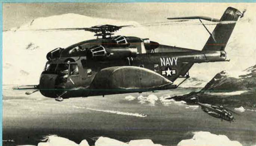
Artist's impression of the fully-developed MH-53E mine-sweeping helicopter, with increased fuel in oversize sponsors
