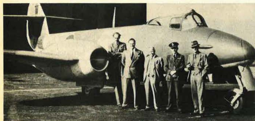
The twin-engine Gloster F.9/40, which finally went into production as the Gloster Meteor. The engine pods were placed in the wings so that development of the airframe could proceed while engine size was finalized. Pictured are (from left): John Crosby-Warren and Michael Daunt, test pilots; Gloster General Manager Frank McKenna; Frank Whittle; and Gloster Chief Designer W. George Carter. (Photo courtesy Gloster Saro Ltd.)
