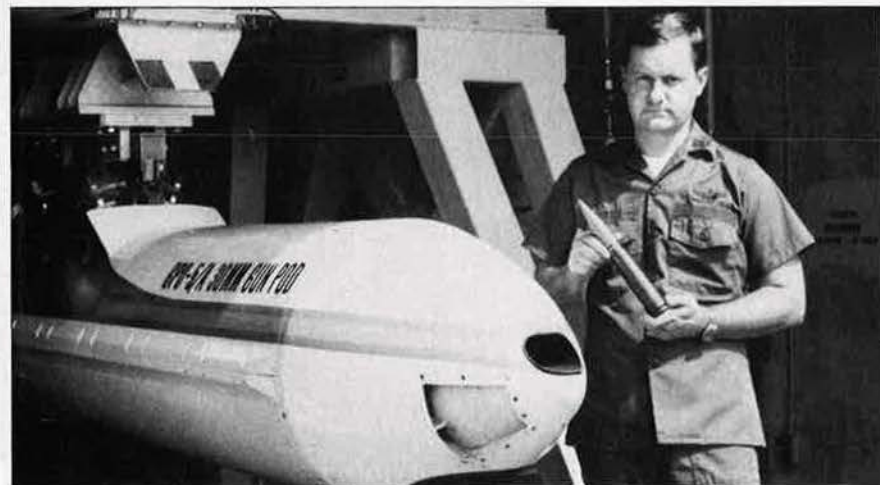
Capt. Ed Zamorski holds a round of 30-mm ammunition that will arm the new GPU-5/A gun-pod system currently under development. See item above.
