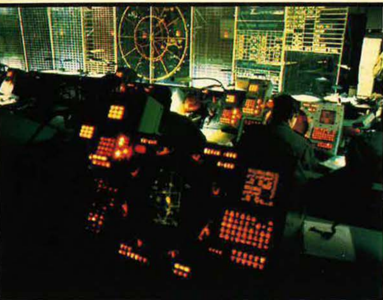
Tactical Air Control Center (TACC), a transportable system about the size of two van-trucks and joined together by an inflatable building. In this area are data-processing equipment, radar displays, and equipment for ground-to-air communications.
