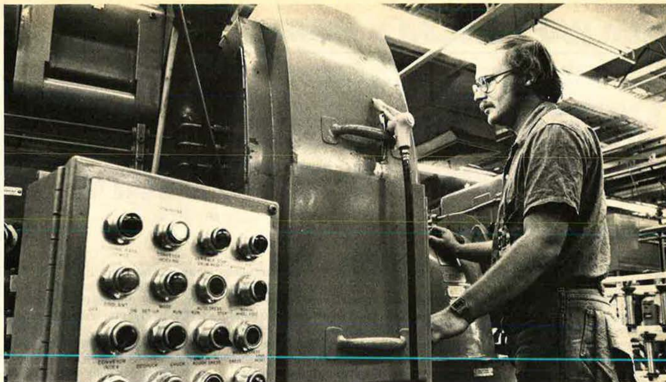
Keith Duckworth, a Garrett machine operator, uses a Curvic Grinder to put curvics on TFE731 engine parts. Curvics, which look like gear teeth, are mated to their counterparts to ensure accurate radial and axial alignment of the engine.
