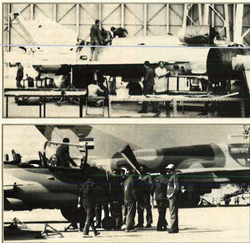
Top, inside the Helwan Depot's Hangar One an EAF MiG-21 undergoes the complete overhaul process, which takes 129 work days per aircraft. Above, an EAF L-29 (foreground) and MiG-21 (background) on the ramp outside Hangar One, undergoing final checkout before acceptance after overhaul. EAF officers consider the overhauled aircraft better than brand-new ones from the factories of origin.
