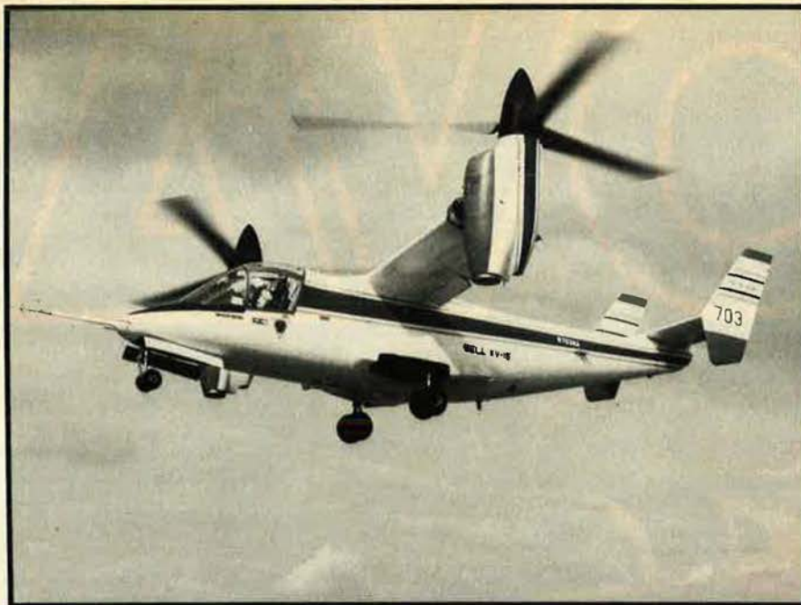
Bell's XV-15 tilt-rotor prototype aircraft, proposed as the basis to meet future transport, close support, medevac, AWACS, ECM, gunship, and other roles. The XV-15 could be the progenitor of an entirely new breed of aircraft.
