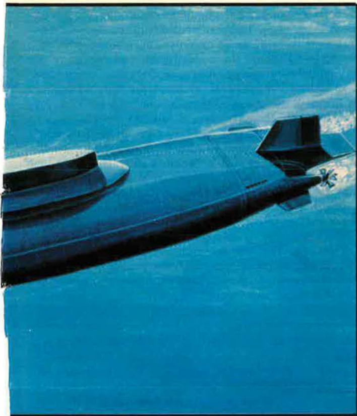
The ultra-modern Typhoon SSBN accommodates twenty of the world's largest SLBMs, each of which can deliver twelve warheads over a distance of 8,300 km with great accuracy.
