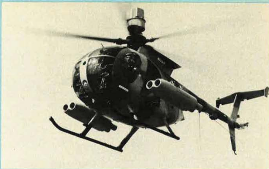
Hughes Model 500MD/MMS-TOW, with mast-mounted sight and TOW anti-tank missiles
