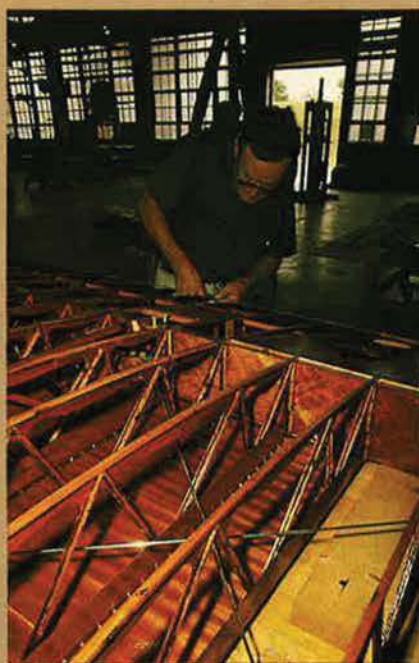
Working from original factory plans and improvising for parts that aren't available anymore, Tom Campbell of the restoration branch crafts the leading edge of a P-26 aircraft wing.
