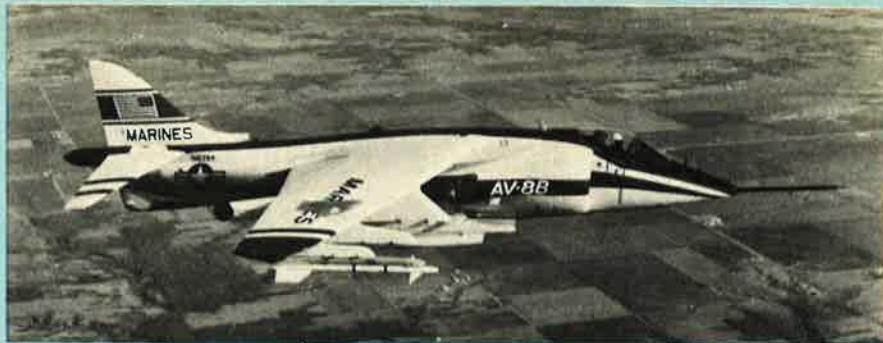
First prototype YAV-8B fitted with wing leading-edge root extensions (LERX) to enhance manoeuvrability
