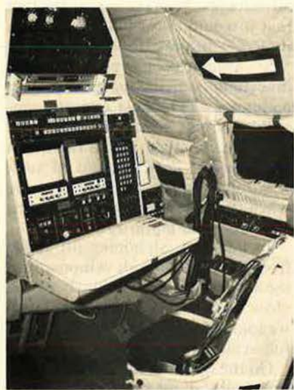
Control console used by ALL's test director to monitor laser operations during the system's test flights.
