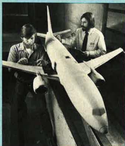
Wind tunnel testing a model of the Boeing 737-300. The repositioned, larger nacelles are clearly evident
