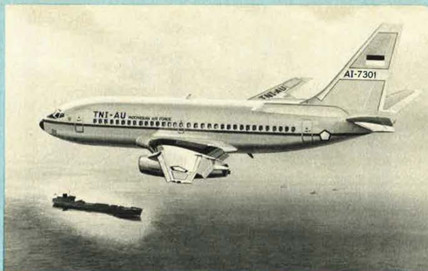
Blade antennae on the top of the rear fuselage identify another new version of the Boeing 737, equipped with Motorola side-looking airborne multi-mission radar (SLAMMR). First order, for 1982-83 delivery, was placed by the Indonesian Air Force, which will use three SLAMMR 737-200s for government transport and maritime surveillance duties
