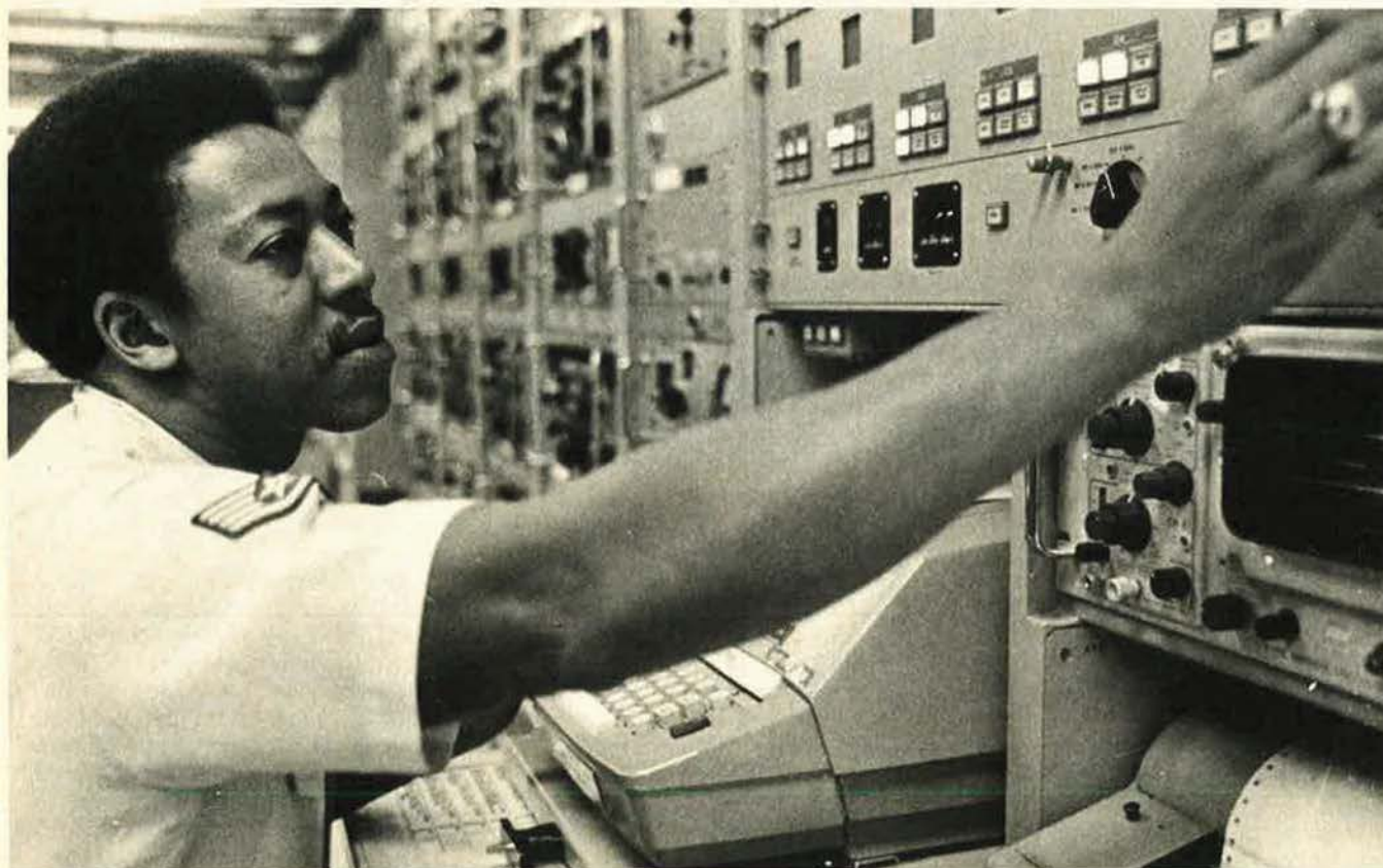
Teleprinter systems are among those areas of communications of vital interest to electronic security experts of all services. The old mechanical printers and keyboards have been succeeded by high-speed electronic hardware.
