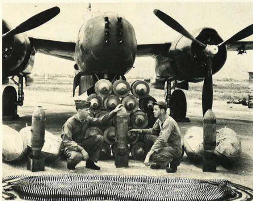
By the time of the Korean War, the Invader had been redesignated B-26 and saw extensive service on night patrols over railways and supply roads in North Korea. Part of the armament the B-26 could carry is shown here, including bombs, .50-caliber ammunition for sixteen guns, napalm tanks, and rockets (not shown).
