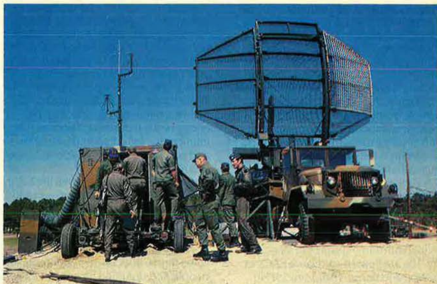
Above, all 507th Wing radar equipment is transportable aboard its own vehicles. Left, the futuristic-looking Air Support Radar Team AN/TPB-1C is capable of directing aircraft to extremely precise coordinates.
