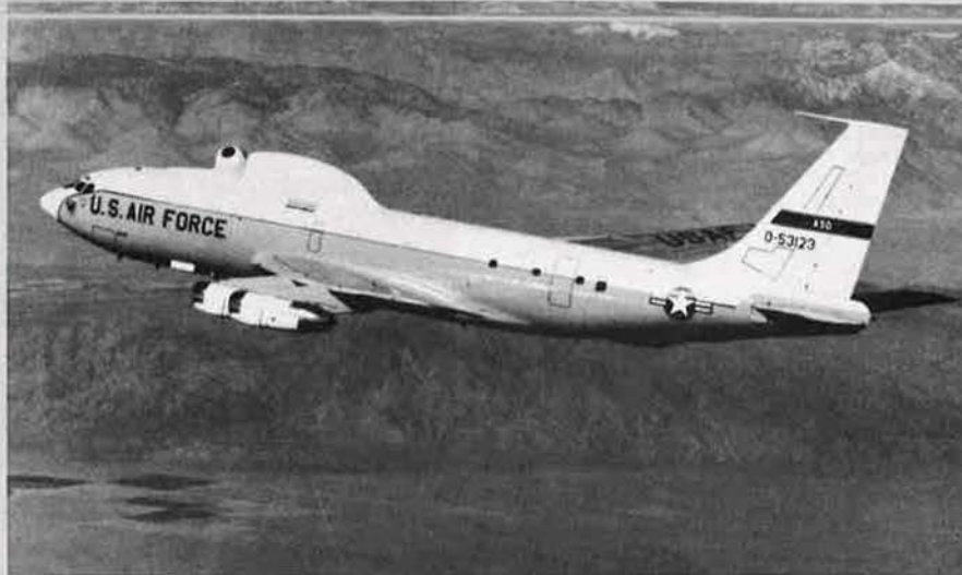
USAF/Boeing NKC-135 airborne laser laboratory, for laser weapon research
