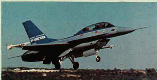
Take-off shots of the two re-engined F-16s, with General Electric J79-GE-119 (left) and F101-DFE engines
