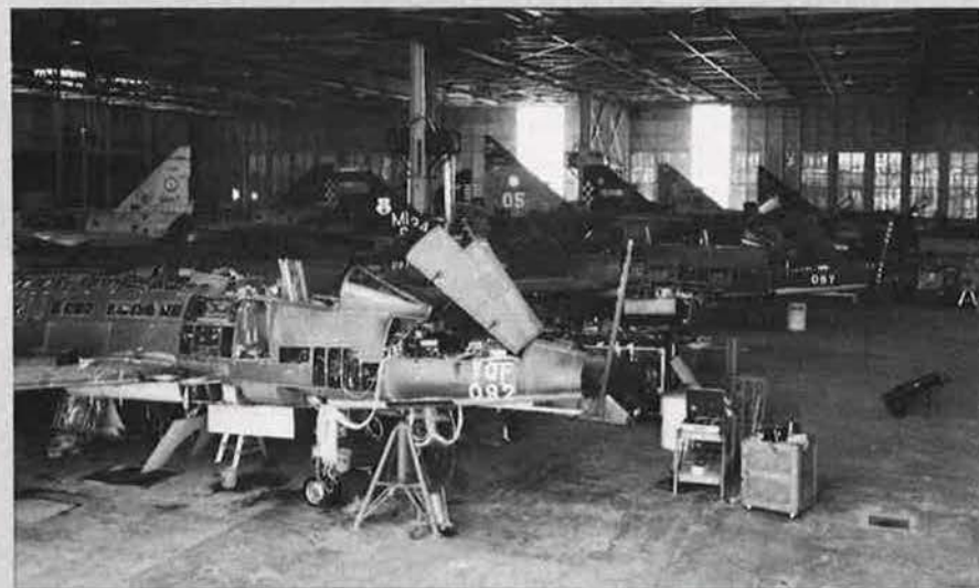
F-100 and F-102A aircraft undergoing conversion to target drone configuration at Sperry's Arizona facility
