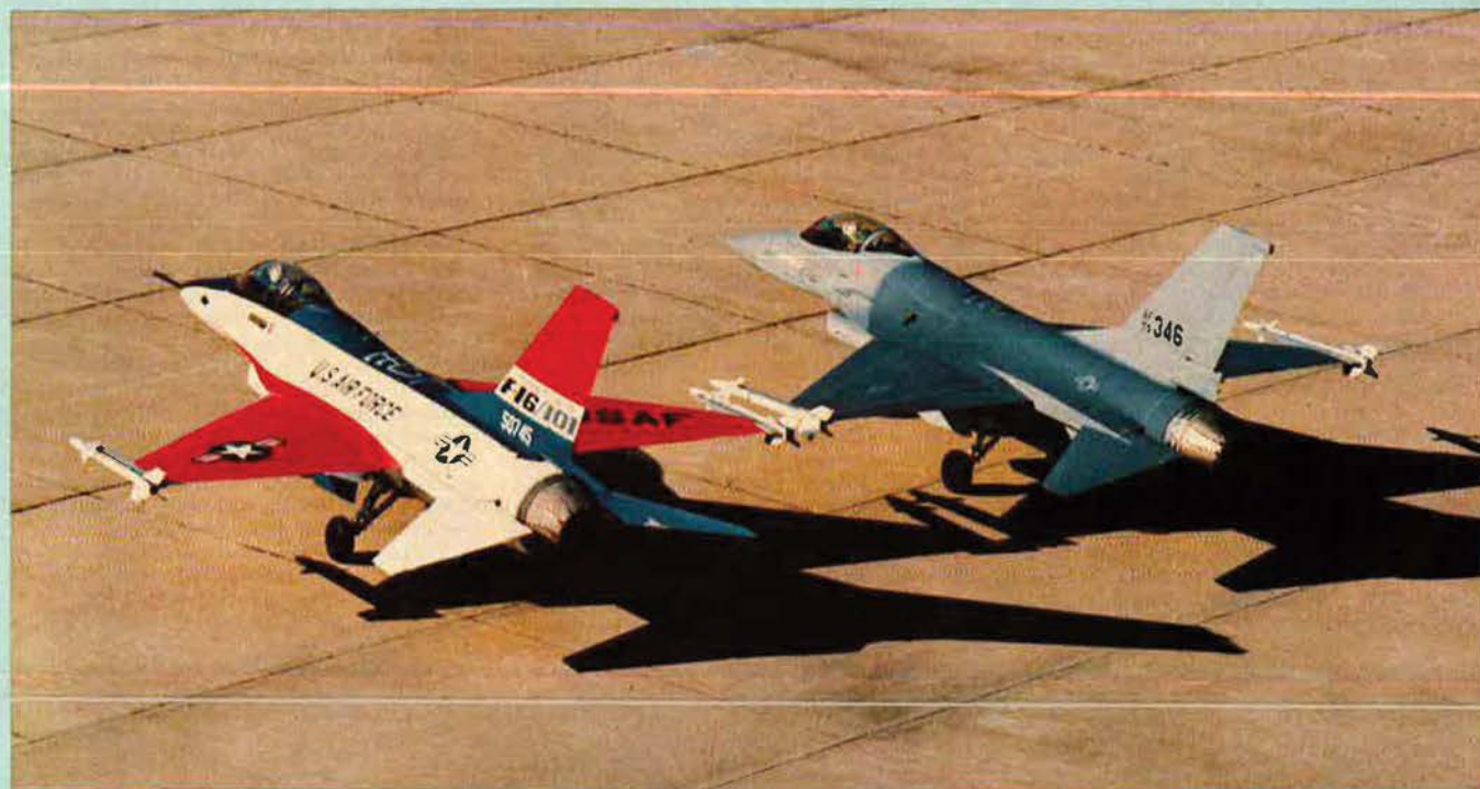
The modest scale of the changes required to re-engine an F-16 with the General Electric F101-DFE derivative fighter engine is emphasised by this photograph. The F-16/101 (left) is almost indistinguishable from the standard F-16A alongside it
