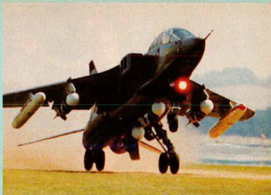
Left, an RAF Jaguar streaks across the British countryside, creating contrails from its passage. Above, rough-field trials included takeoffs and landings from such sod strips as this one at Boscombe Down test center.
