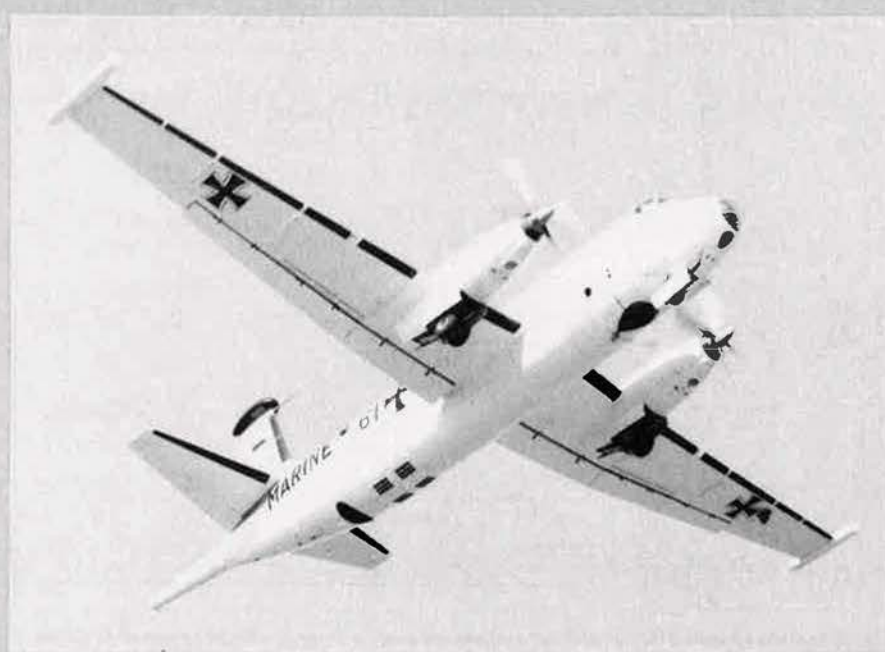
Wingtip ESM pods help to identify this German Navy Atlantic as one of the first to be updated by Dornier
