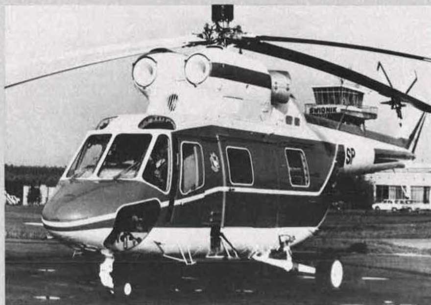
PZL Swidnik W-3 Sokół, a 12-passenger helicopter developed from the Soviet-designed Mi-2
