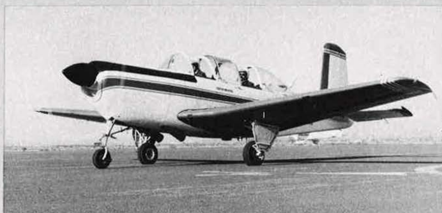
Marsh Turbo Mentor turboprop conversion of the Beechcraft T-34 primary trainer
