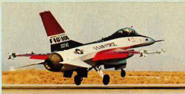
Take-off shots of the two re-engined F-16s, with General Electric J79-GE-119 (left) and F101-DFE engines
