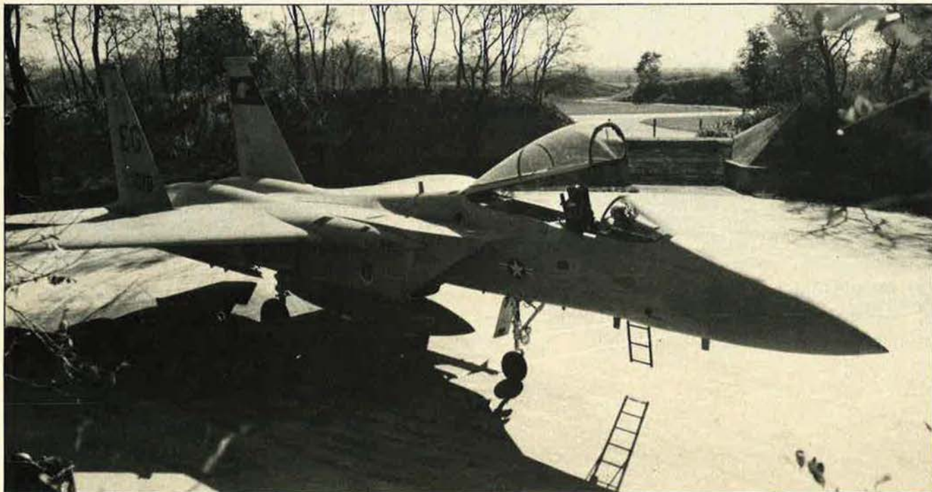
F-15 Eagles participating in the recent twenty-day exercise dubbed Coronet Eagle required minimum ground-support personnel, as each aircraft is equipped with on-board starting and power sources and a boarding ladder.
