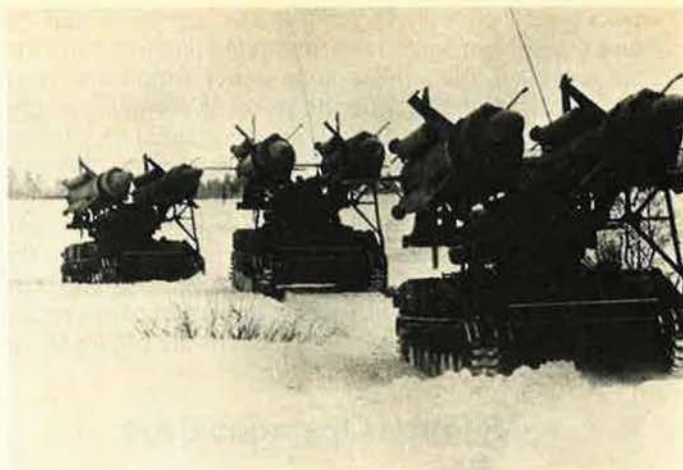
The SA-4 Ganef anti-aircraft missile's ramjet propulsion gives it a slant range of forty-three miles.
