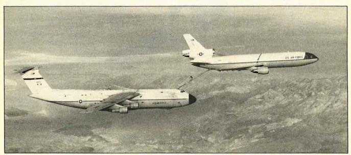
An Air Force KC-10A built by McDonnell Douglas hooks up with a C-5 transport over Edwards AFB, Calif., in the first test refueling of the tanker and the first test of the aircraft's advanced aerial refueling boom.
