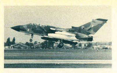
Marconi's new and very advanced ECM pod under the wing of an RAF Tornado. Known as Sky Shadow, the pod is typical of new equipment being developed for this key aircraft.
