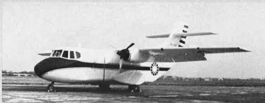
AIDC XC-2 prototype twin-turboprop transport, under development in Taiwan
