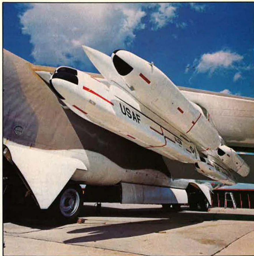
Shapes designed to simulate the AGM-109 (top) and AGM-86B have been used to test the flight characteristics of a new B-52 ALCM wing pylon.
