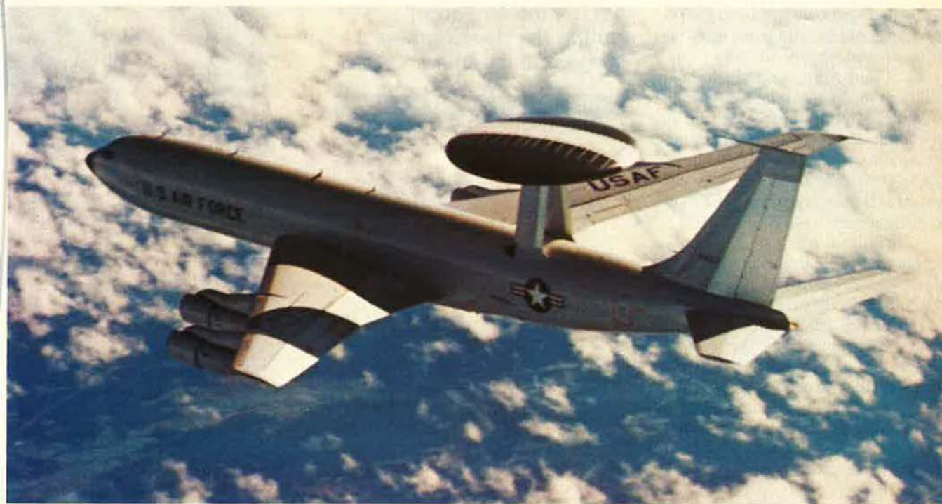
Distinctive rotodome, housing radar antennas and associated equipment, identifies the modified Boeing 707-320B as an E-3A.
