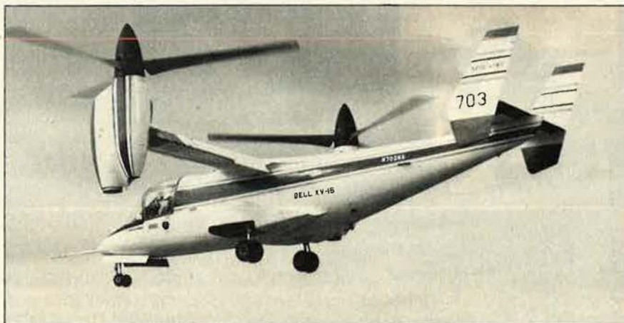
The second of two XV-15s built by Bell Helicopter Textron under US Army/NASA sponsorship. Conversion from helicopter to airplane flight mode is expected during tests later this year, when a safe operating envelope will be established and performance, dynamic stability, and handling qualities evaluated.
