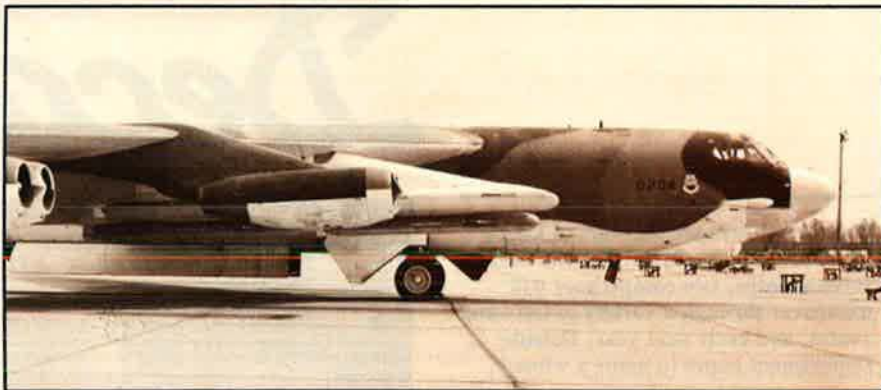
In addition to launches from the B-52 bomb bay, AGM-86s (top) and AGM-109s will be released from pylons on the B-52 wings.
