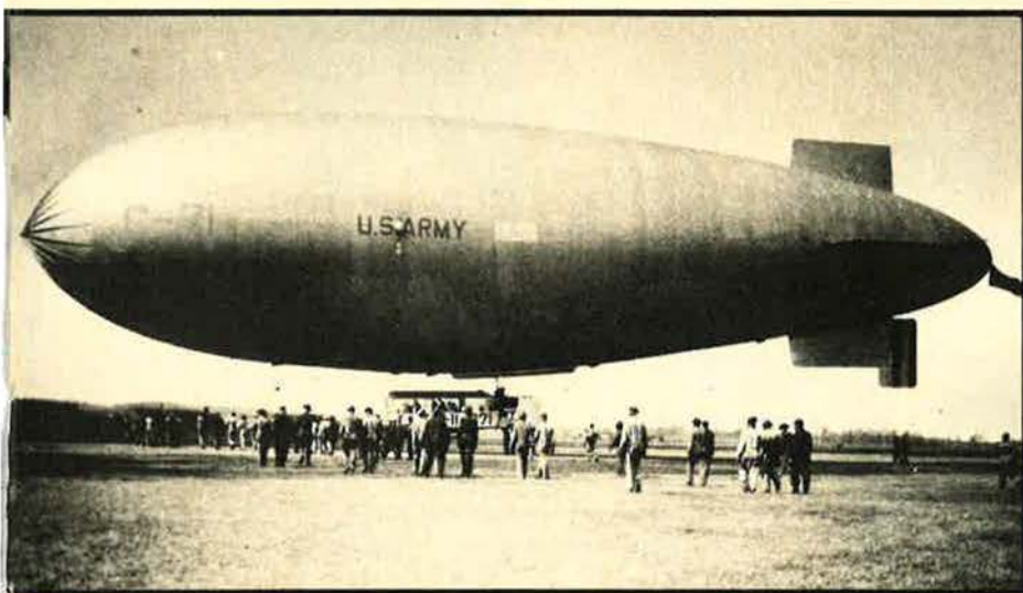
Shortly before World War II, the Army balloon program had progressed to this C-7 nonrigid, helium-filled vehicle equipped with a four-place, twin-engine gondola. When war came, these were transferred to the Navy for patrol duties.
