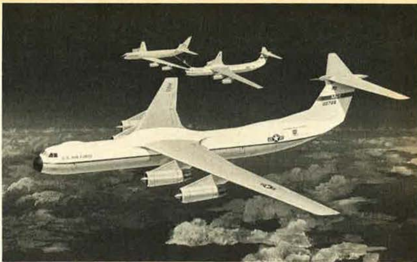
A key element in increasing US strategic aircraft capabilities is "stretching" the C-141 StarLifter through the addition of a 23.5-foot-long fuselage extension depicted in this artist's conception. The C-141 is air-refuelable.
