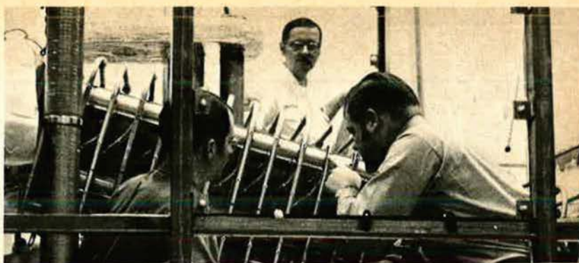
Lab personnel look over the two-million-volt Marx Generator, built entirely in house. It will be used to simulate the electromagnetic-pulse (EMP) effects of a nuclear explosion.
