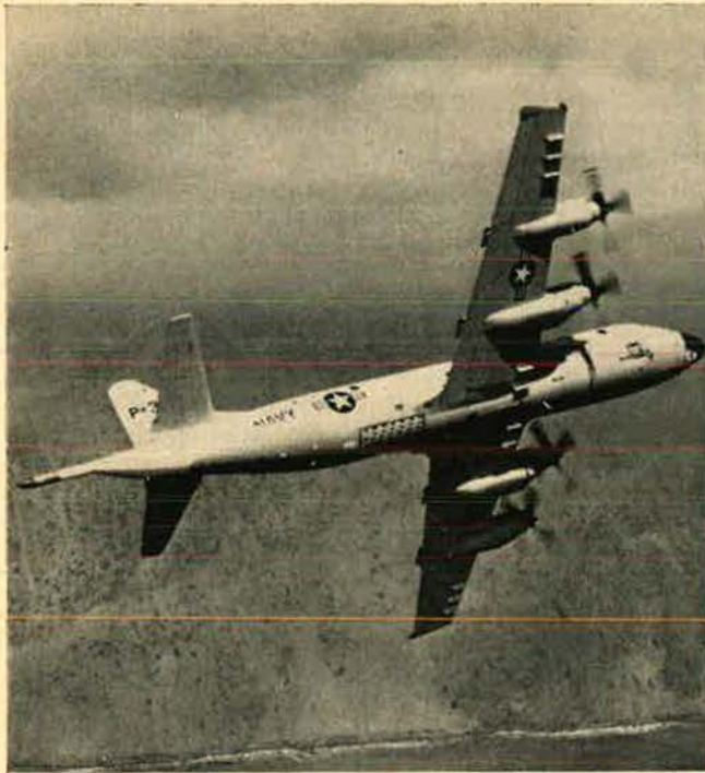
The P-3C version of the Orion submarine-hunting aircraft. Upgraded from the A and B models, the P-3C has fifty-two sonobuoy launch tubes and an integrated general-purpose computer to speed up and simplify ASW procedures.
