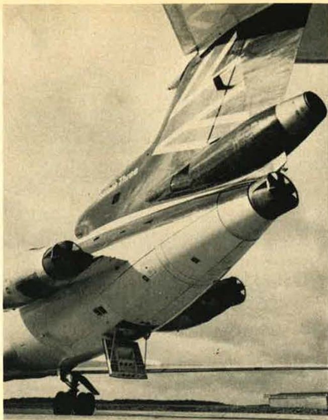
This is a closeup of the booster engine in the tail of the Trident 3B. When it is used, it permits the three other engines to operate below maximum and cuts noise output.
