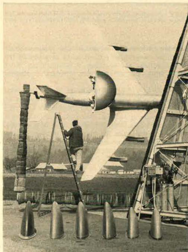
Distinguishing feature, and most critical component of AWACS, is 30-foot-diameter, externally mounted radome, housing down-looking radar to find and track enemy planes.
