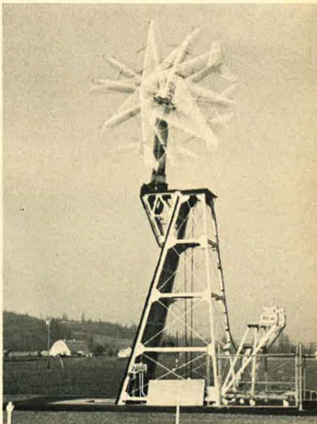
AWACS model moving on a mobile test tower at Boeing's Seattle Radome Laboratory. AWACS's complex antenna system requires seventy-five high-powered antennas.
