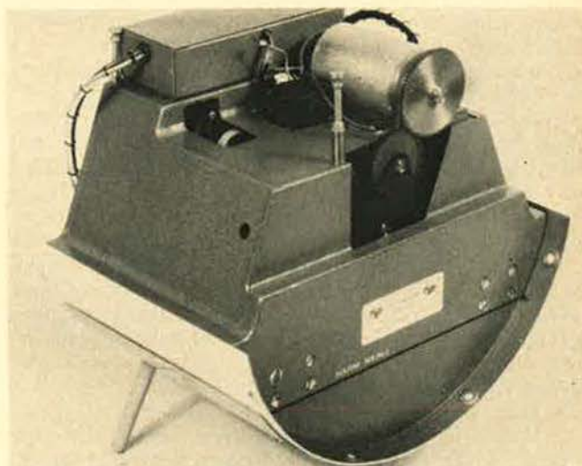
The Hawker Siddeley Dynamics infrared linescan system is a sensor that will be used in a new surveillance drone.
