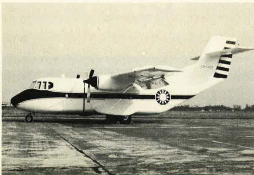
The XC-2 twin turboprop transport prototype is powered by Lycoming T-53 engines, which are also used in the T-CH-1 trainer.
