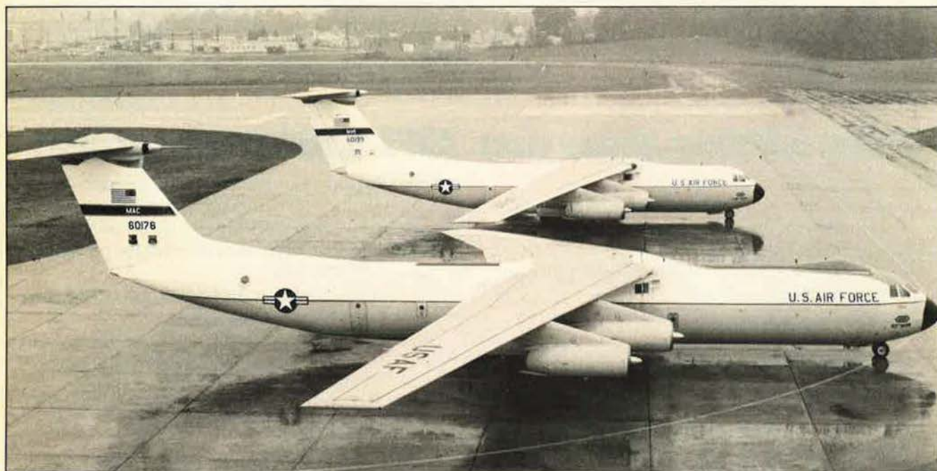
A comparison of the "stretched" C-141B transport, foreground, and the original "A" version. The first modified StarLifter, to be stationed at Charleston AFB, S. C., was delivered to the Military Airlift Command in December. When the program to modify the entire fleet of 217 C-141s is concluded in 1982, MAC will have gained cargo capacity equivalent to an additional ninety of the jet transports. Another significant airlift advantage will be the aircrafts' aerial-refueling capability. With a payload capacity of forty tons, the stretched C-141 will serve as MAC's airlift workhorse in the 1980s.
