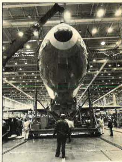
The first KC-10A Advanced Tanker Cargo Aircraft is undergoing assembly at the McDonnell Douglas plant in Long Beach, Calif. Delivery of the aircraft to the Air Force is expected by year's end.
