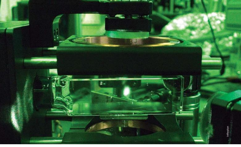
A Rubidium cold-atom cloud, visible as the central bright spot in this infrared image, is captured at the intersection of laser beams in a trapped atom vacuum system. Laser cooling plays a crucial role in quantum applications.
