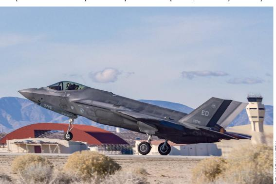
An F-35A took off from Edwards Air Force Base, Calif., in January, conducting the first flight of an F-35 with the complete Technology Refresh 3 (TR-3) suite of updates. The upgrade adds the computer and electrical power to support a range of long-promised Block 4 capabilities.
