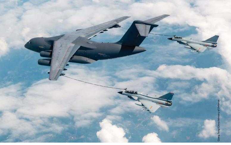
China has rapidly modernized its air force, with iterative generations of fighter aircraft. A YY-20 tanker refueled two J-10 fighter jets in July. The J-10 is an indigenous design, part of China's drive to be self sufficient as its own high-end weapons supplier.
