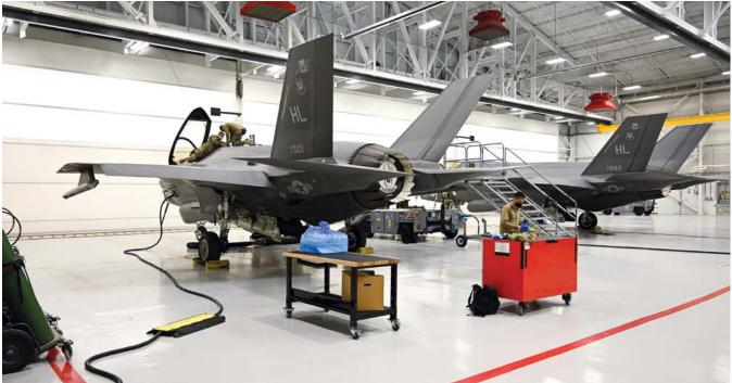
Maintainers with the 421st Fighter Generation Squadron care for F-35A Lightning IIs at Hill Air Force Base, Utah. The jets' engines must generate electric power to run advanced sensors and computer systems and provide cooling to keep those systems from overheating. Coming upgrades will demand even more power and cooling.
