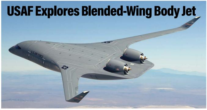
JetZero, a Long Beach, Calif, startup, will build the Air Force a KC-46-size blended-wing body flight demonstrator. The concept allows 30 to 50 percent range gains versus tube-and-wing aircraft and will inform future tanker or airlifter designs.
