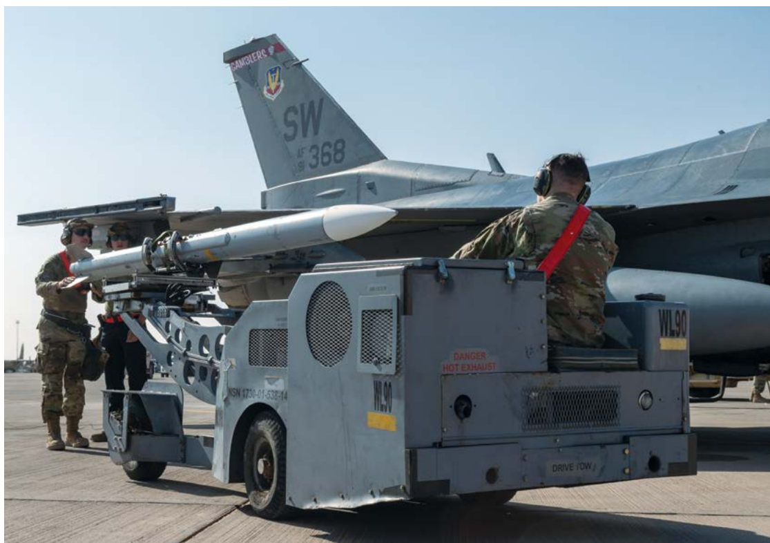
Airmen assigned to the 77th Expeditionary Fighter Squadron, prepare to load an AIM-120 advanced medium-range air-to-air missile (AMRAAM) on an F-16 in November at Prince Sultan Air Base, Saudi Arabia. For Western airpower aid to Ukraine, it's not just a question of the aircraft. They must be paired with modern air-to-air missiles, such as the AIM-120 AMRAAM, to be effective.
