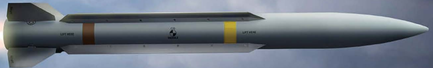
Raytheon's Peregrine is a compact, high-speed air-to-air missile for countering drones, cruise missiles, and manned aircraft. Designed for affordability, the weapon's light weight effectively doubles the number of missiles fighters can carry.
