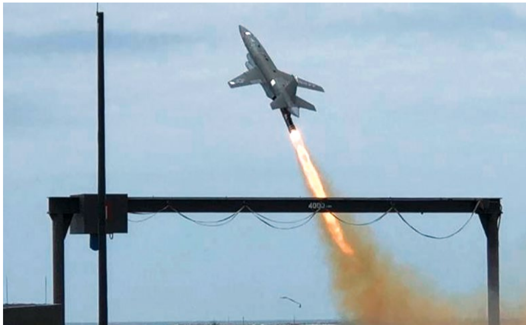
The Skyborg autonomy core system launches aboard a Kratos UTAP-22 tactical uncrewed vehicle at Tyndall AFB, Fla. The aim of the Skyborg program is to integrate full-mission autonomy with low-cost, attritable uncrewed air vehicle technology to enable crewed-uncrewed teaming.
