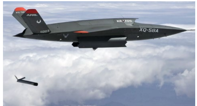
The unmanned XQ-58A Valkyrie releases the ALTIUS-600 small unmanned aircraft system in a test at the U.S. Army Yuma Proving Ground test range, Ariz., March 26, 2021.
