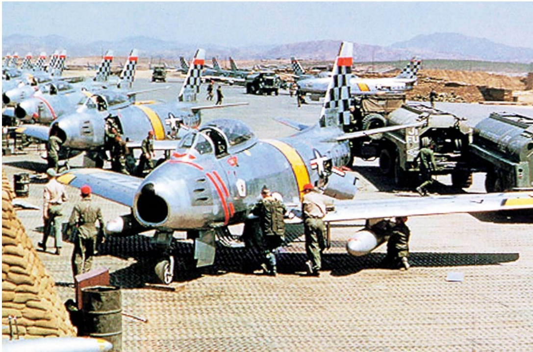
North American F-86 Sabre fighter jets are readied for combat during the Korean War at Suwon Air Base, South Korea. Note perforated steel mats. Steel mats allowed some aircraft to successfully use degraded and decaying runways at South Korean air bases.
