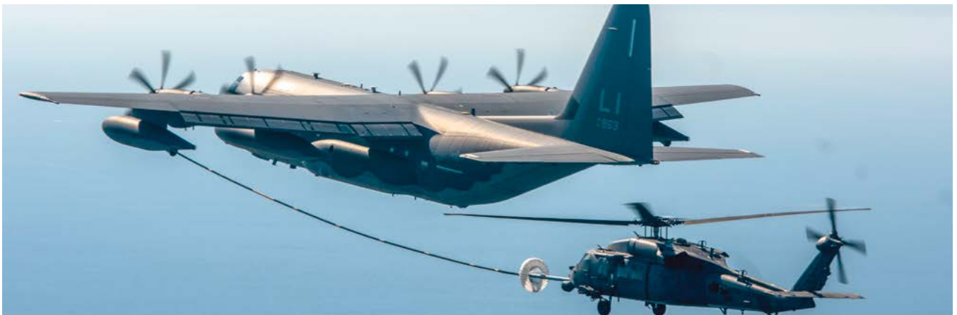
An HC-130J refuels an HH-60G Pave Hawk helicopter during a combat search and rescue training event at Osan Air Base, South Korea.
