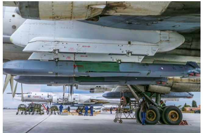
Russian Kh-101 nuclear-armed air-launched conventional long-range, standoff cruise missiles are mounted on Tu-95MS Bear bombers at an undisclosed location.
