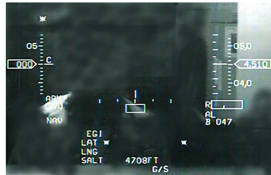
Figure 9: Simulated PFD and HUD in INS OFF Position (Tab T-18)
