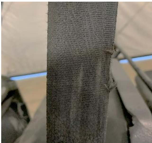
Figure 19 – Fraying on MV Seatbelt (Tab Z-29)
