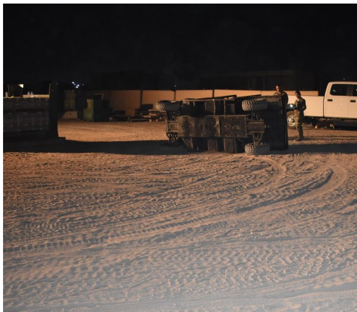
Figure 9 – MV's Tire Tracks While Attempting Left Hand Turn (Tab S-5)
