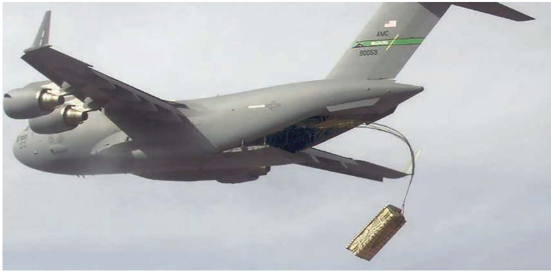
A high-altitude airdrop of simulated Joint Air-to-Surface Standoff Missiles on a pallet demonstrates how a C-17 Globemaster III airlifter could in the future be used to launch weapons using airdrop procedures.
