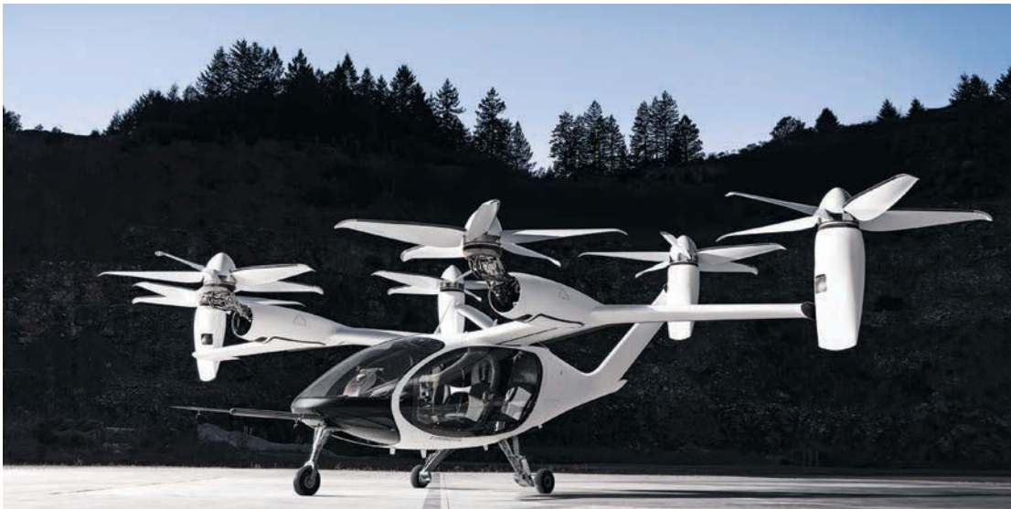
Joby Aviation's eVTOL aircraft has six rotors and seats five, including the pilot. It can take off vertically, like a helicopter, and then shift into forward flight using tilt-rotors. Joby says it can reach a top speed of 200 mph, can travel 150 miles on a single charge, and is 100 times quieter than a conventional aircraft.
