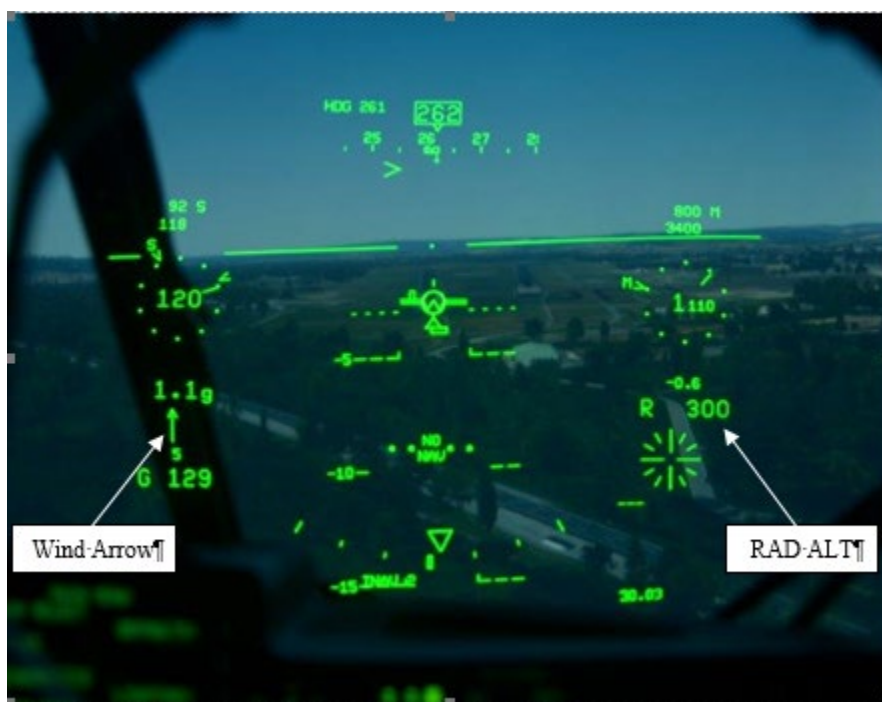
Figure 5: C-130J HUD highlighting the wind arrow and RAD ALT at 300 feet AGL (Tab DD-XX)
