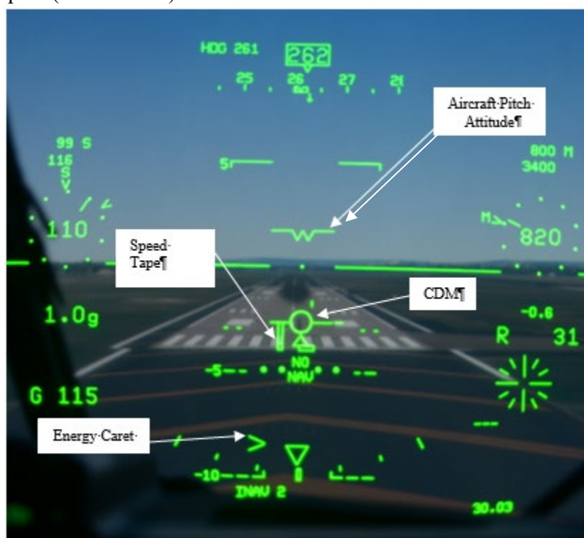
Figure 28: HUD of the WST with highlighted references at 31 feet AGL after mimicking the mishap throttle position and maintaining aim point (Tab DD-26)
