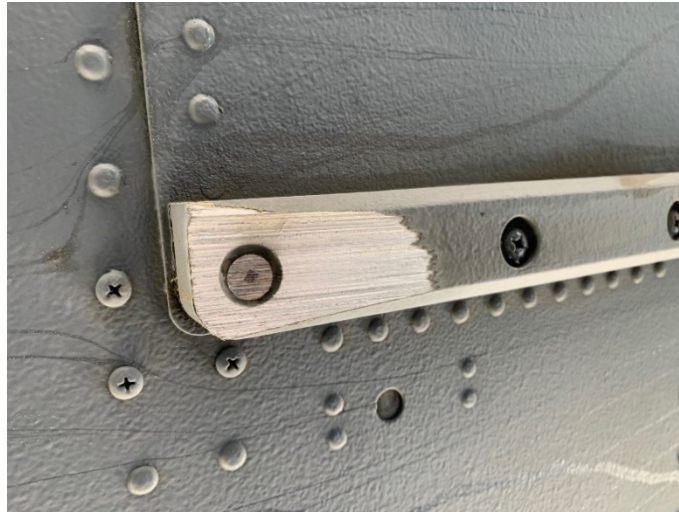
Figure 18: Right Hand Tail Skid Plate Impact Damage (Tab S-7)
