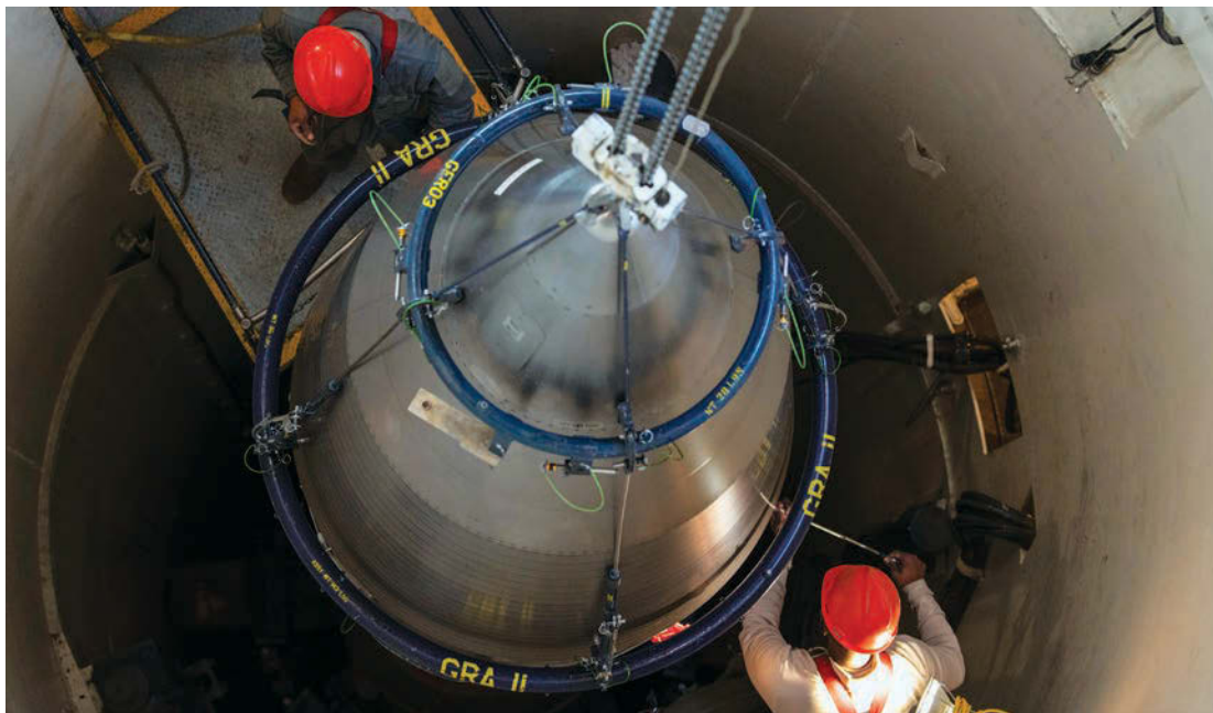
Minuteman III nuclear missiles, which replaced Peacekeeper missiles in the 1970s, will in turn be replaced by the Ground-Based Strategic Deterrent, which won’t enter service until 2029. Here, Airmen maintain a 50-year-old Minuteman III at the F.E. Warren missile complex in Wyoming.
