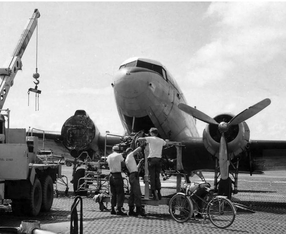
Maintainers work on an SC-47 atop a steel runway at an undisclosed location. The aircraft was a C-47 transport modified to drop flairs, supplies, and leaflets.
