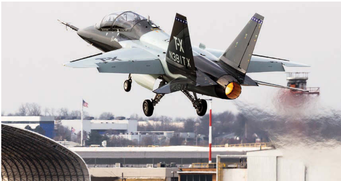
In 2017, a T-X with afterburners flies in tests in St. Louis. Now dubbed the T-7 Red Hawk, in tribute to the Tuskegee Airmen, the Boeing/Saab aircraft will replace the T-38 as USAF’s premier fighter trainer.
