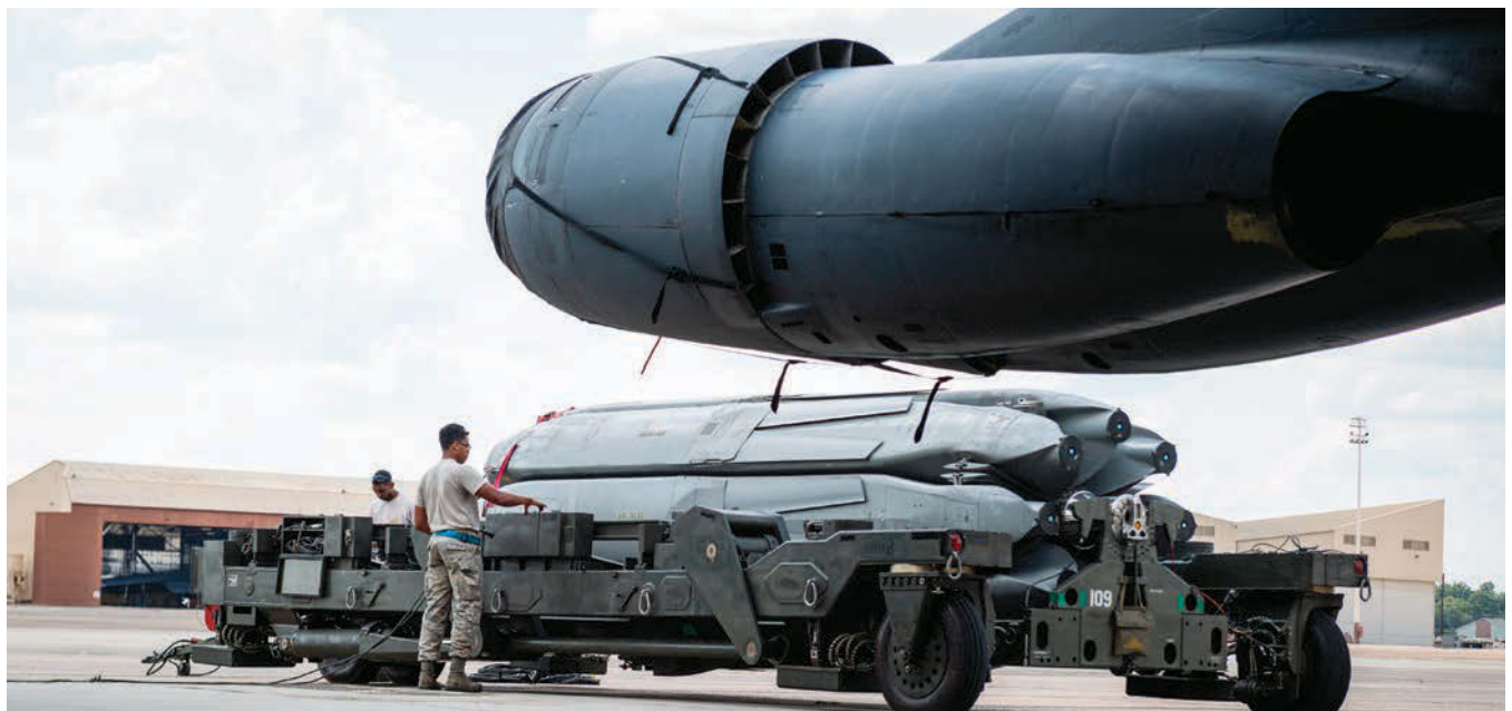
A crew readies a Common Strategic Rotary Launcher full of AGM-86B ALCMs for loading onto a B-52H at Barksdale AFB, La. The ALCM is long past its planned retirement and will be succeeded by the highly secret AGM-181 Long-Range Standoff missile. Upgrades will allow other smart weapons to be carried internally.
