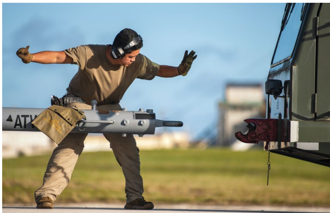
Senior Airman Jae Sajonas, 9th Expeditionary Bomb Squadron B-1B Lancer assistant crew chief, helps align an MB-2 Tow Tractor on the flight line at Andersen Air Force Base, Guam, May 14. Tow tractors are used to bring aircraft to their parking locations.
