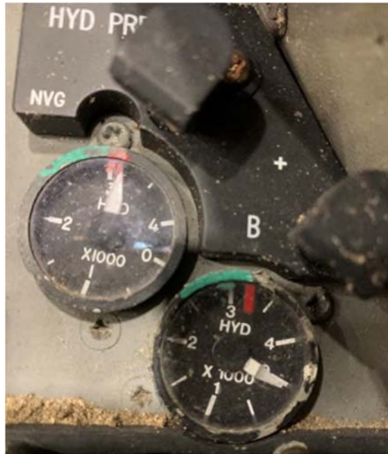
Image 11. Post-mishap Hydraulic System Pressure Gauges (Tab Z-9)
