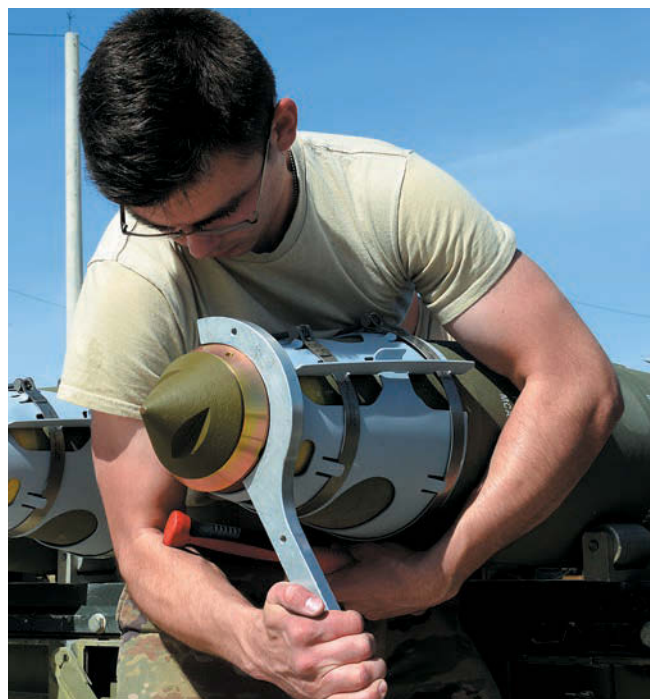
SrA. Ethan Dietz tightens the nose extender on a GBU-36 JDAM at Kandhar Airfield, Afghanistan. GPS-guided munitions are being used in Iraq, Syria, and Afghanistan.
