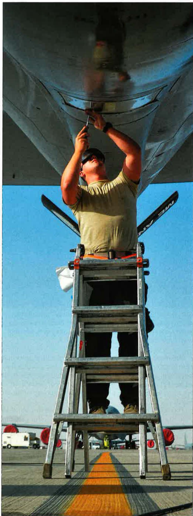
At Al Udeid AB, Qatar, a 340th Aircraft Maintenance Unit maintainer adjusts the window of a KC-135 boom pod before a flight for Operation Inherent Resolve. Al Udeid is one of 20 bases Davis' squadron team is visiting to solicit feedback from airmen.
