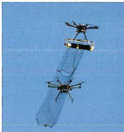
An attack drone demonstrates part of a counter-unmanned aerial system: a net.
