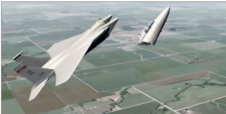
Image from a video produced by Boeing as part of the Air Force's accident investigation reconstructing the in-flight structural failure of an ANG F-15C in November 2007. The breakup was caused by fatigue cracking of a forward fuselage longeron; the pilot survived.
