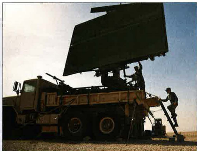
SrA. Joseph Fletcher and A1C Christopher Kelly of the 71st Expeditionary Air Control Squadron prepare to inspect a TPS-75 radar. 3DELRR is a follow-on to this radar.
