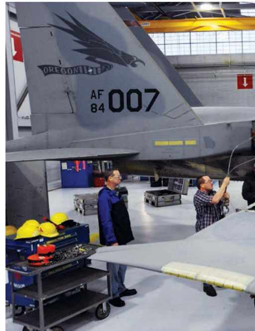
Contractors remove the wings from an F-15 at Portland Arpt., Ore. When sequester was applied in full force two years ago it led to a backlog of maintenance from which USAF still has not recovered.
