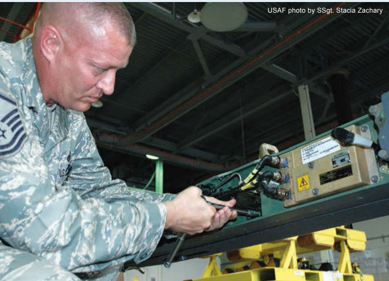
MSgt. Brian Mosier adjusts an SDB II pneumatic carriage system used to mount the weapon on the aircraft.
