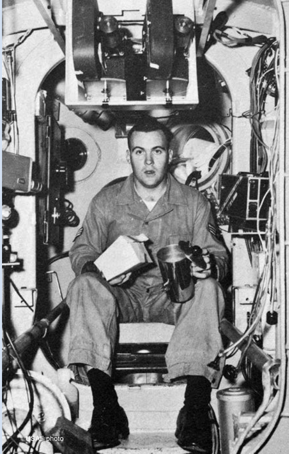
A1C Donald Farrell takes a meal in the “imitation spaceship” built by the Air Force School of Space Medicine to test the effects of space travel on the human body. During the actual test, Farrell spent a week in the cramped capsule.
