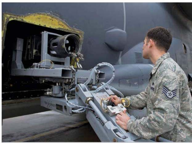
Roll Out the Barrel: SSgt. Ronnie Simons, a weapons load team chief, inserts a 25 mm Gatling gun into an AC-130U Spooky gunship at Hurlburt Field, Fla., Jan. 12. The guns are inspected and the barrels switched out every 18,000 rounds.
