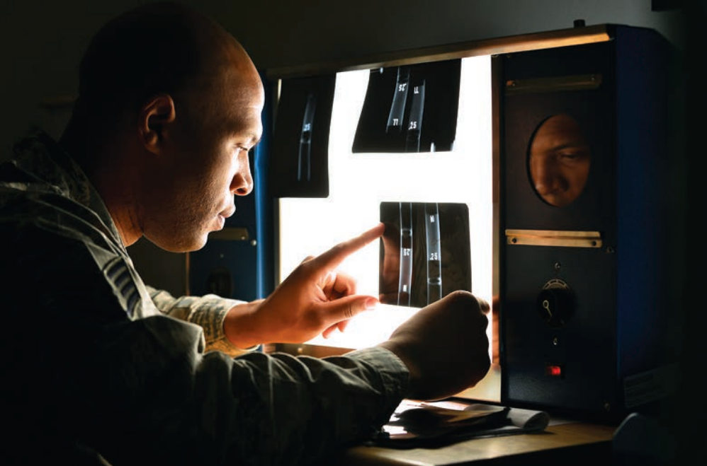
SSgt. Robert Eady inspects X-ray images of foreign object damage discovered in an aircraft. Even tiny bits of debris can lead to disaster if introduced to an engine during flight.
