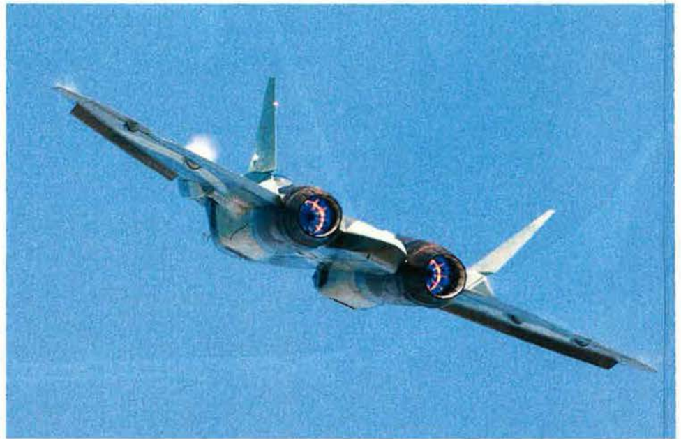
Russia's T-50 has thrust-vectoring engines, claimed to be capable of supercruise. Russia and India may build roughly 400 T-50s together and offer more for export.
