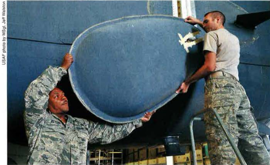
TSgt. Edward Ector (l), 5th Maintenance Squadron, hands SSgt. John Slaughter (r), 307th Maintenance Squadron, a radio transmitter radome at Minot AFB, N.D. Both Ector, who is Active Duty, and Slaughter, a Reservist, are communications navigation systems technicians.
