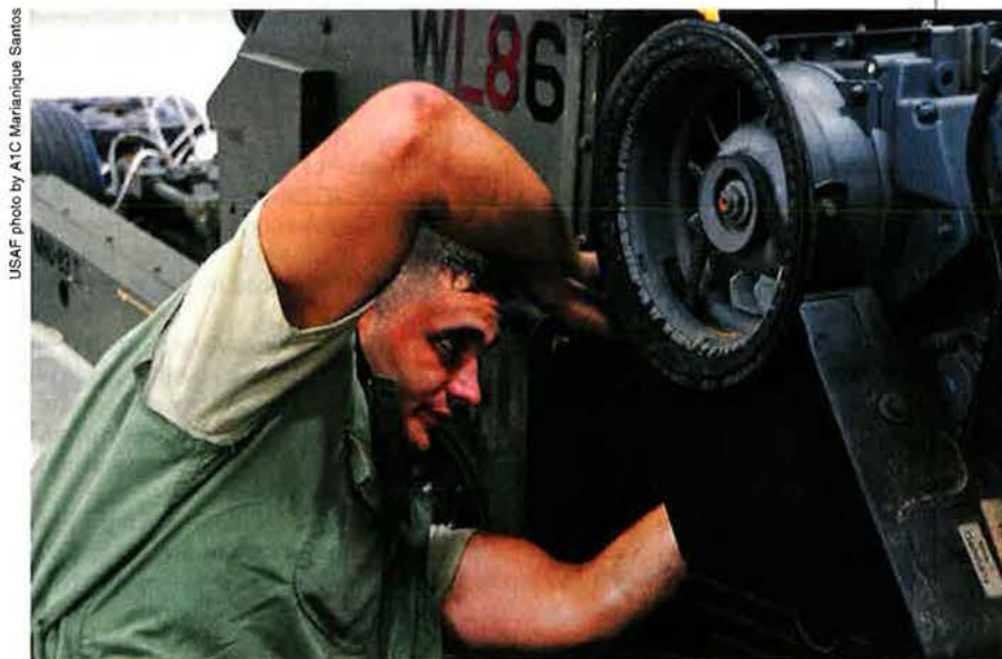
A Little Change in the Weather: A1C Andrew Caprio, deployed from JB Elmendorf-Richardson, Alaska, to Andersen AFB, Guam, replaces fuel lines on a munitions handling unit used for B-52 weapon loading. Maintainers are busy on the flight line at Andersen, and the work is especially challenging because they must quickly become accustomed to the shop and procedures.
