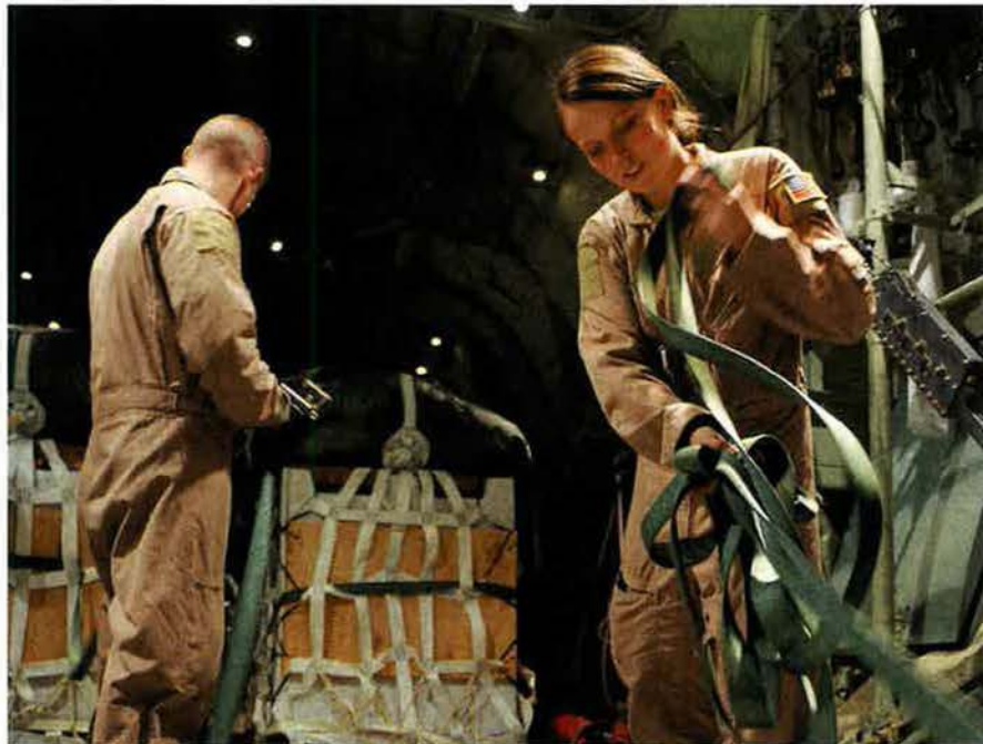
Tie Me Kangaroo Down, Sport: SSgt. T. J. Grover (l) and A1C Rachael Orazine ready straps used to secure airdrop bundles in the belly of a C-130J at Kandahar Airfield, Afghanistan. Both airmen are loadmasters with the 772nd Expeditionary Airlift Squadron. Loadmasters run preflight checks of the aircraft, make sure all equipment is working, supervise cargo and passenger loading, and calculate the weight and balance of the load.
