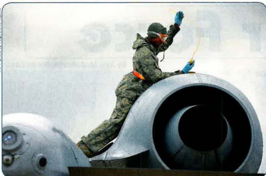
A1C Tevin Duhart checks for debris in an oil sample taken from an A-10 engine at Selfridge ANGB, Mich.
