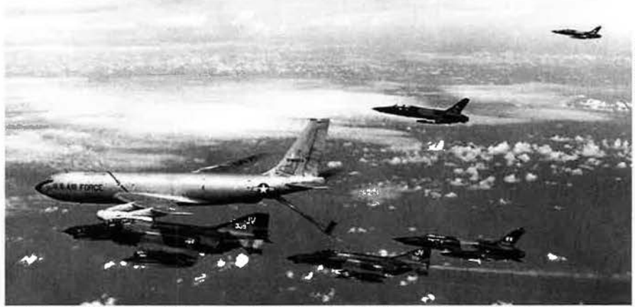
A USAF SAM hunter-killer group including two F-4Es and three F-105Gs takes turns refueling from a KC-135 during a Linebacker mission.
