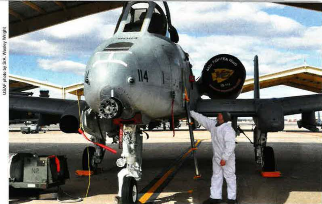
Amn. Branden Jewell closes the canopy of a 442nd Fighter Wing A-10 after loading the aircraft with liquid oxygen at Whiteman AFB, Mo. Air Combat Command began exploring the idea of associations in the A-10 community in 2002.
