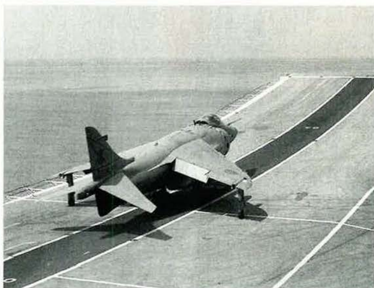
A Sea Harrier uses a ski-jump bump while taking off from HMS Invincible .
