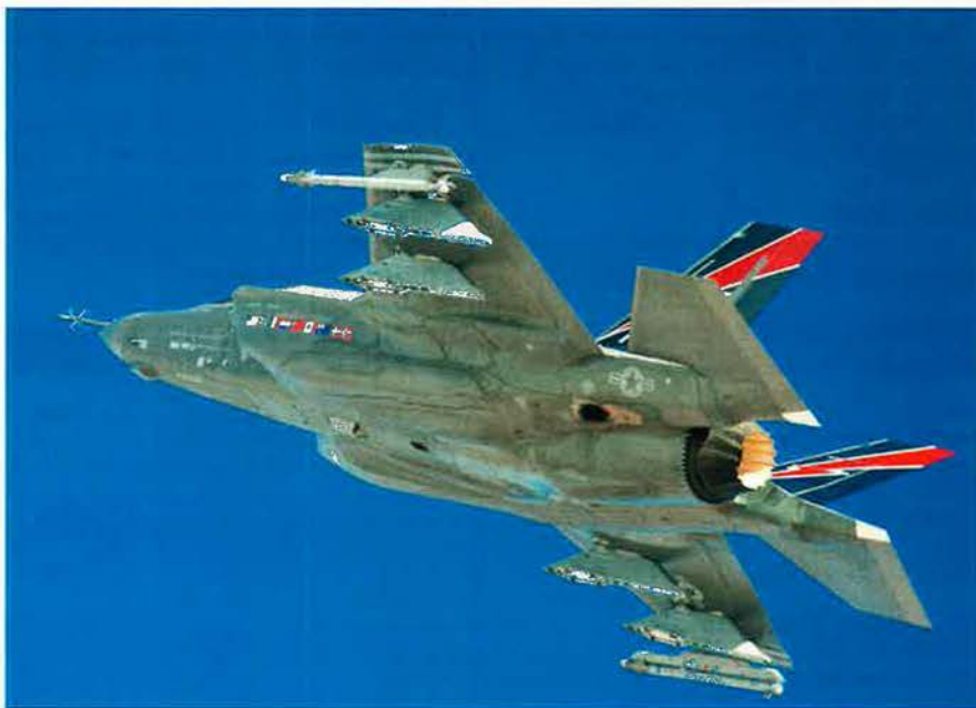
On the Wing: An F-35A flew the type's first external weapons test mission at Edwards AFB, Calif., Feb. 16. The test aircraft carried two air-to-air AIM-9X missiles on outboard wing stations and internally hauled two 2,000-pound GBU-31 guided bombs and two advanced medium range AIM-120 air-to-air missiles.
