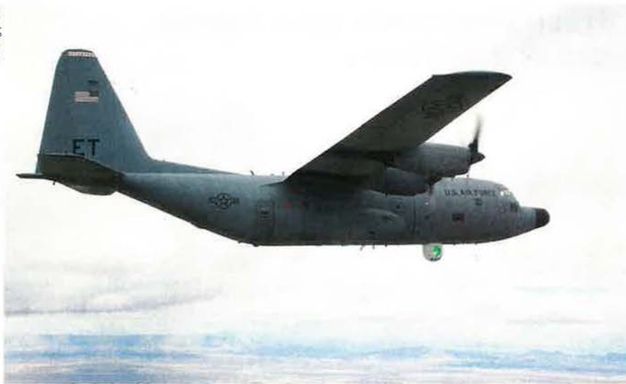
The Advanced Tactical Laser system aircraft—a modified C-130 transport—proved a laser system could be effective against certain ground targets, but has been shelved.
