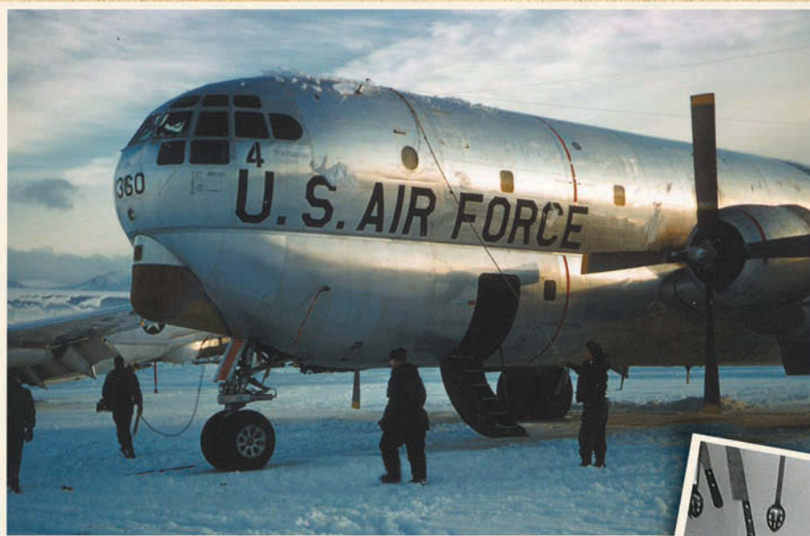
Navigator 1st Lt. Richard Heitman took this 1957 photo showing snow removal from 93rd Air Refueling Squadron KC-97s, deployed from Castle AFB, Calif., to Elmendorf AFB, Alaska. The crew threw a knotted rope over the tanker's fuselage. Airmen on each end of the rope pulled it back and forth along its length. Retired Lt. Col. Heitman is from the Palm Springs Chapter, Calif.
