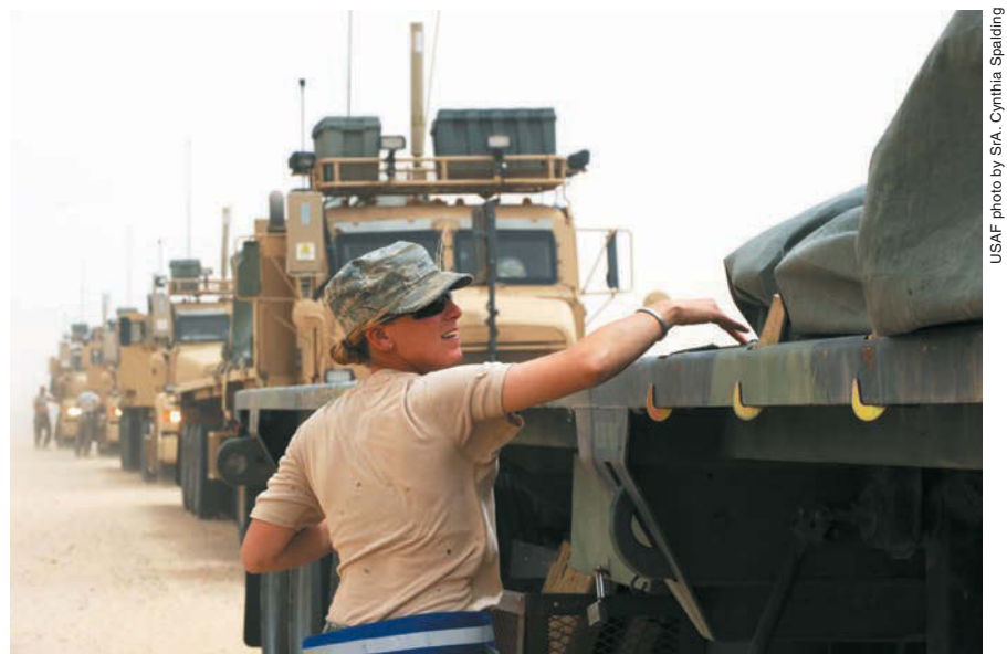
Tied Up Tight: SrA. Kelly McLain, a vehicle operator with the 387th Expeditionary Logistics Readiness Squadron, takes advantage of a quick roadside stop to check the cargo tarp and straps during a convoy mission. Making sure cargo is fully secured cuts down on unscheduled stops in a hostile environment.
