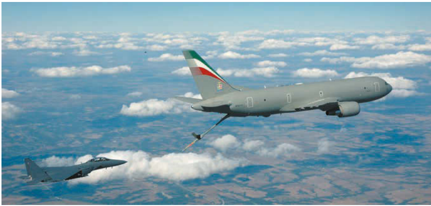
The KC-46A will be derived from Boeing's 767, shown here in Italian Air Force livery with an F-15. New features will include both boom and probe-and-drogue refueling systems.
