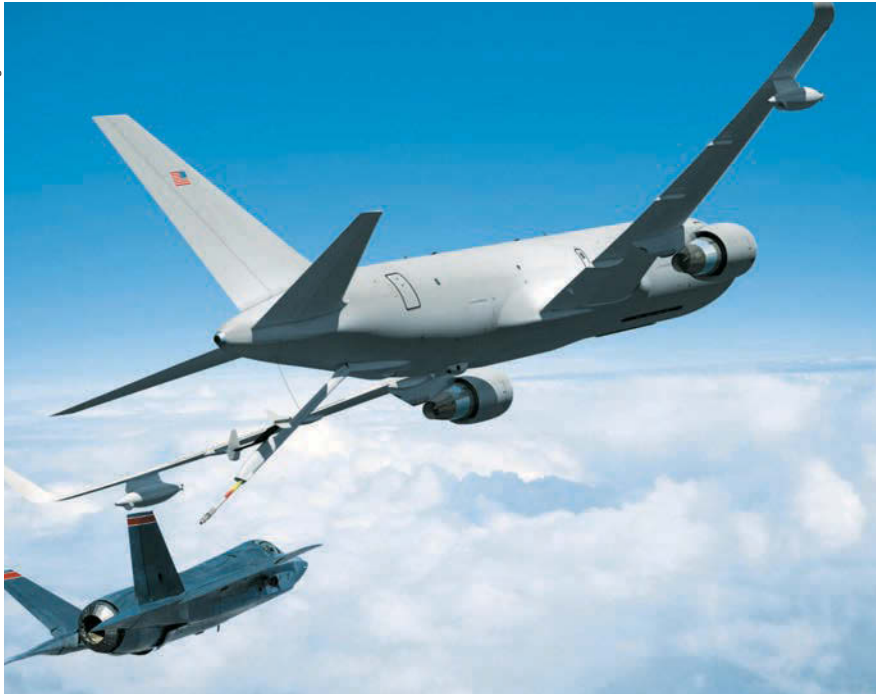
An F-35 prepares to refuel from a KC-46A in this Boeing graphic. To simplify the KC-X competition, USAF specified an airplane very much like its existing KC-135.
