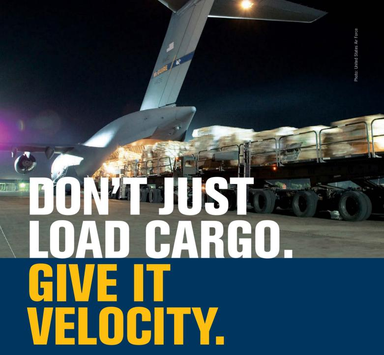
With a 30-ton capacity and the ability to precisely control height (up to 18.5 feet) as well as pitch and yaw, the Tunner from DRS is a high-tech workhorse that can unload and load a C-17 with amazing accuracy and speed. Plus, two or more Tunners can be used together to create a cargo bridge for even greater volume and productivity. **Velocity In Cargo Loading: That's Go To.**
