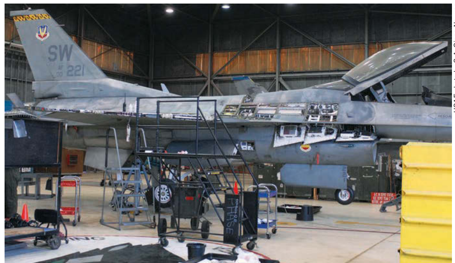
An F-16 is put through its every-400-hours phase inspection. The service lives of some F-16s will have to be extended to accommodate delays in F-35 delivery.
